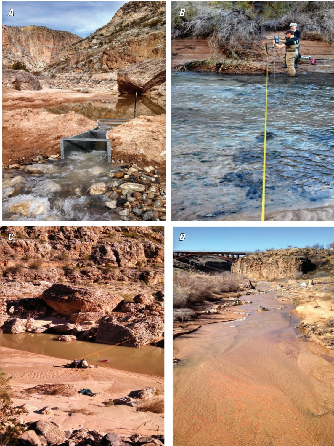
Figure 7. Virgin River discharge measurement sites during the Pah Tempe Springs interference tests. A , upstream of the Pah Tempe Springs reach at PTVRU during the low-flow tests of November 2013 and February 2014, using a Parshall flume, B , downstream of the springs reach at PTVRL using a SonTek FlowTracker Handheld Acoustic Doppler Velocimeter® (ADV), C , upstream of the springs reach at PTVRU during the high-flow test of November 2014 using a Teledyne RD Instruments StreamPro acoustic Doppler current profiler (ADCP), and D , downstream of the springs reach at PTVRL. Shifting sand channel with collapsing banks prevented development of a reliable stage-discharge relation.
