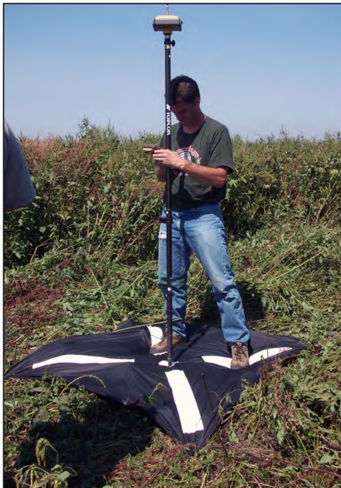
Figure 8. Surveying a target used to georeference images from the drone. Photograph by Kathleen Neitzert.
