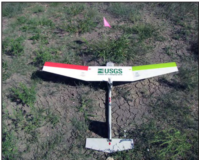
Figure 7. A small, unmanned aerial system (drone) used to collect imagery data of the shoreline near Lower Brule, South Dakota. Photograph by Kathleen Neitzert.
