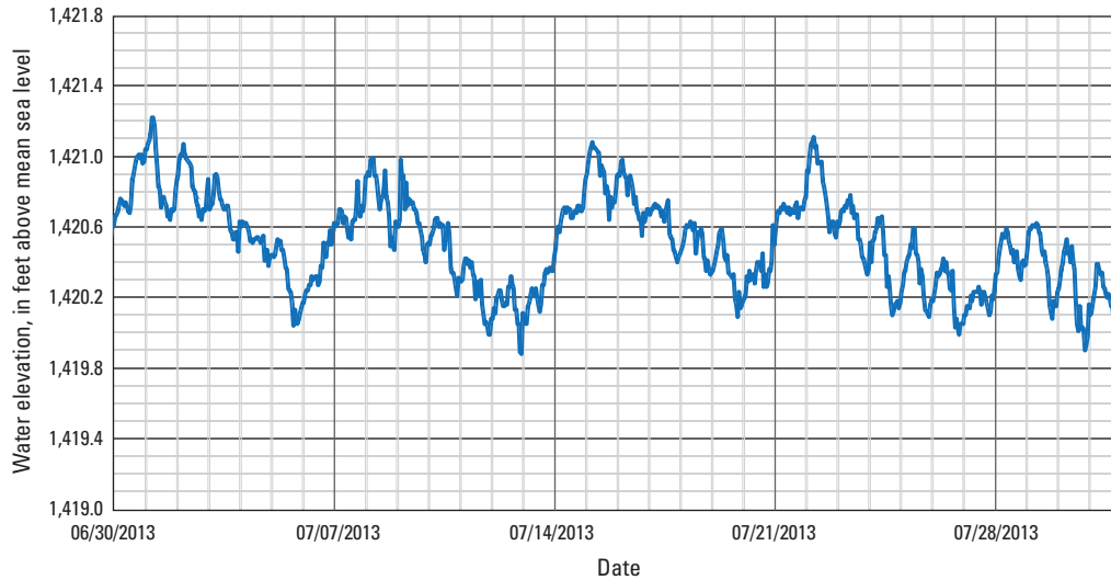
Figure 11. Hourly reservoir water elevation data for July 2013 on Lake Sharpe, South Dakota.
