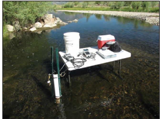
Figure 7. Water-quality sonde deployment at stream site East Fork Carson River near Muller Lane downstream transect (SDT), East Fork Carson River, Carson Valley, west-central Nevada.
