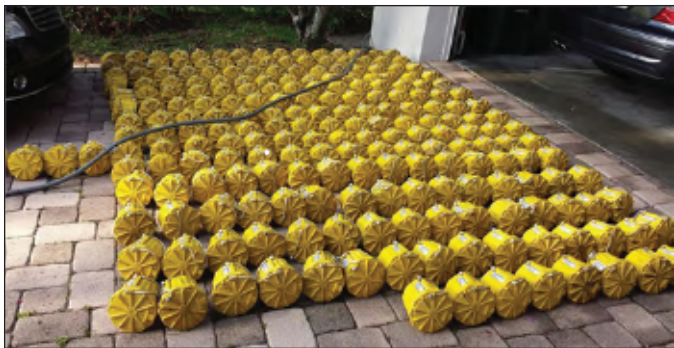
Figure 4. Geospace GCX1 autonomous nodal receivers used for the acquisition of the three-dimensional (3D) seismic surveys for this study.
