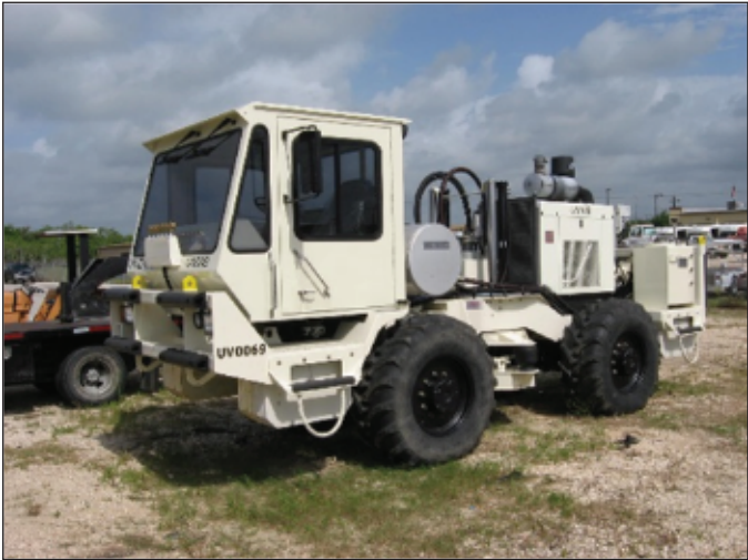
Figure 3. Inova Univib vibrator used in acquisition of the three-dimensional (3D) seismic surveys for this study.
