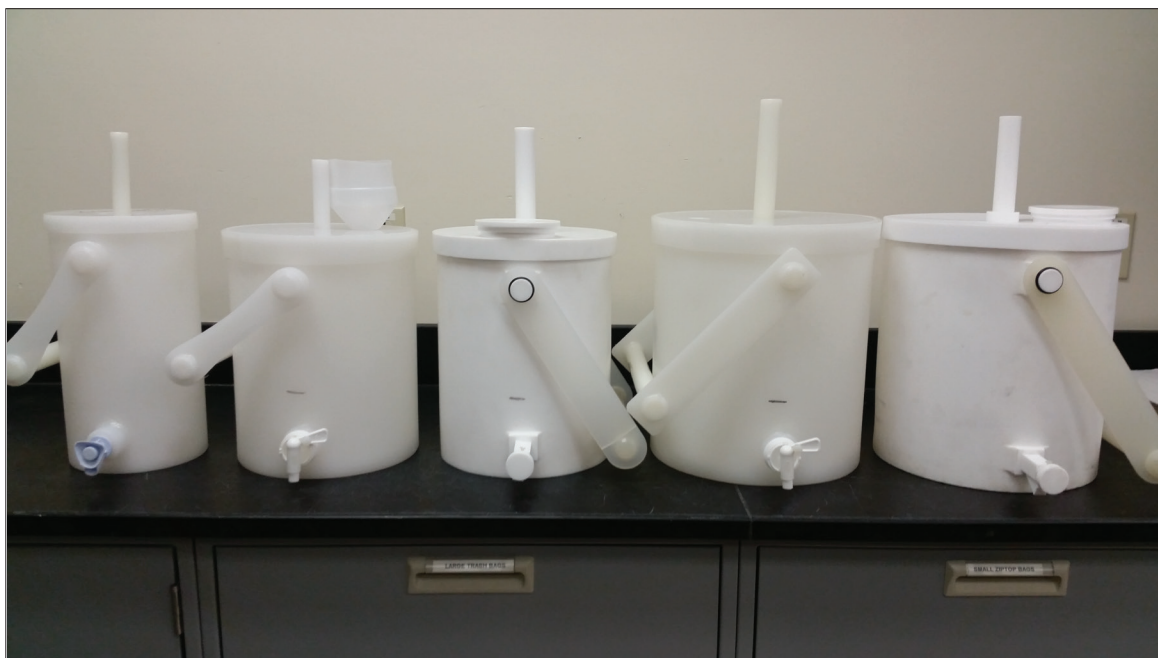
Figure 1. Photograph showing all churn splitters used in the study from left to right: 4-liter polyethylene with cooler-type spigot, 8-liter polyethylene with (all-plastic) cubitainer-style spigot, 8-liter fluorocarbon polymer with fluorocarbon-polymer spigot, 14-liter polyethylene with cubitainer-style spigot, and 14-liter fluorocarbon polymer with fluorocarbon-polymer spigot.
