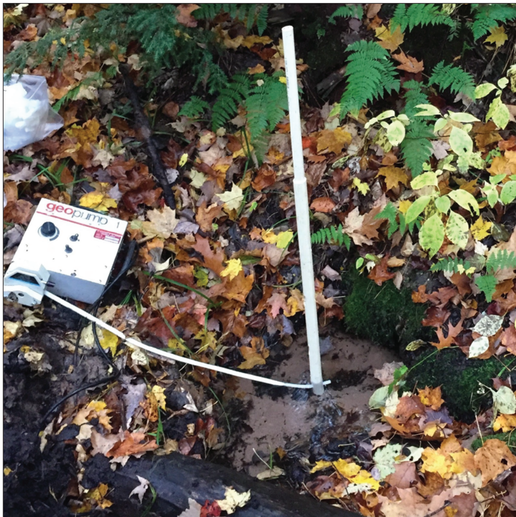
Figure 4. A, spring sampling apparatus and B, example of spring sample collection at U.S. Geological Survey station 464545087522801.
