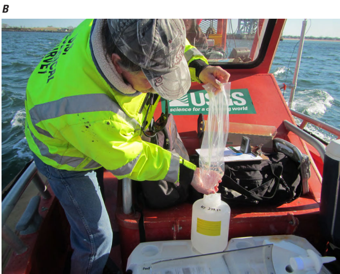
Figure 8. The collection of depth-integrated, equal discharge increment samples of suspended-sediment concentration: A, D-96-A1 sampler, and B, transferring water from sample bag into polyethylene bottle. Photographs by U.S. Geological Survey.
