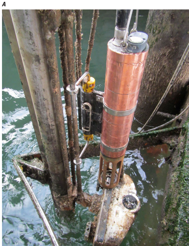
Figure 5. A water-quality monitor with antifouling measures: A , monitor body with copper tape and brass probe guard and B , copper-taped monitor bulkhead, brass turbidity probe, and copper mesh over conductivity/temperature probe. Photographs by R. Cartwright, U.S. Geological Survey.
