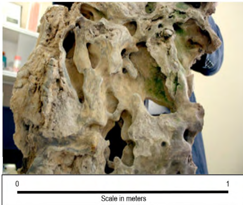
Figure 6. Weathered slab of chert showing voids where limestone was completely dissolved, illustrating the three-dimensional lobate shape of the two different lithologies that formed the couplets. This contact is interpreted as being pre-induration of the silica gel and the carbonate sediment. Planar contacts are thought to have been indurated and thus more rigid. Orientation of slab shows underside of bedding plane.
