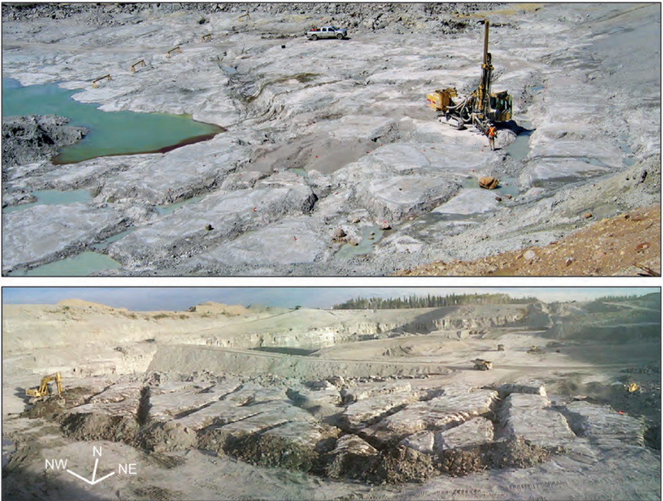
Figure 7. Solution-enlarged joints in the Moberly Member limestone, Waterways Formation (Devonian), exhumed at the Hammerstone Quarry, western Bitumount Trough. The 2- to 3-meter-deep joints were solution-enlarged at the water table and extend downward as narrow 10- to 15-centimeter-wide filled joints. Joint fills of insoluble residues are removed during quarrying to facilitate use of the limestone as crushed rock for road construction. Modified from Broughton (2018c, 2019).
