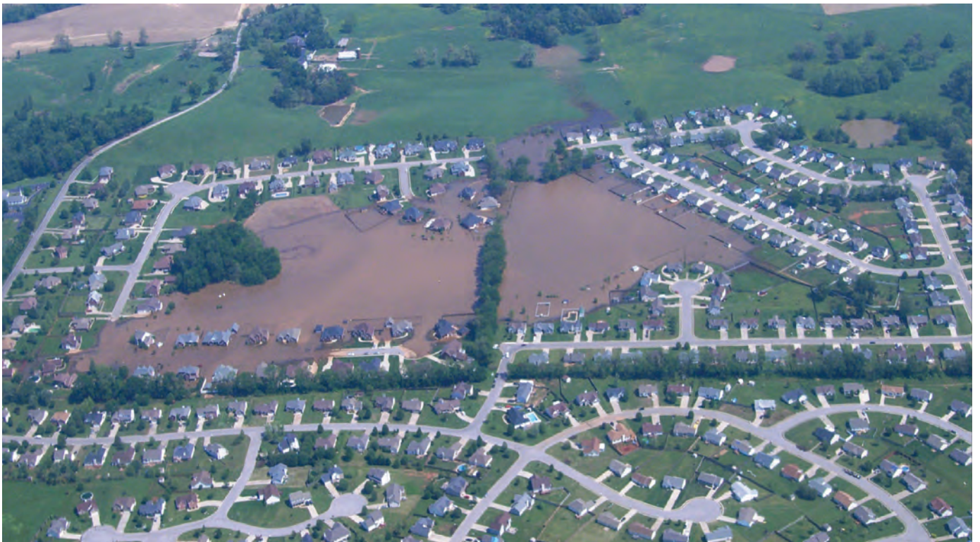
Figure 5. Aerial view of sinkhole flooding at a subdivision underlain by the St. Louis Limestone near Clarksville, Tennessee, in the northern Highland Rim. Photograph taken May 5, 2010, by M. Bradley, U.S. Geological Survey.
