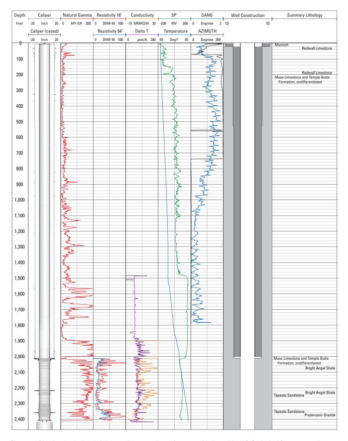
**Figure 8.** Plot showing the borehole logs, well construction, and summary lithology of the U.S. Geological Survey test well, western Hualapai Plateau (Hualapai Test Well on figure 1), northwestern Arizona. Ohm-meters, OHM-M; spontaneous potential, SP; millivolts, MV; delta time, Delta T; microsecond per feet, µsec/ft; degrees Fahrenheit, Deg F.
