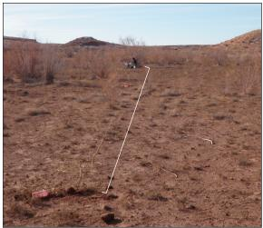
**Figure 6.** Diagram (*A*) and photographs (*B, C*) showing controlled source audio-frequency magnetotelluric setup used to study the western Hualapai Plateau, northwestern Arizona. Diagram modified from Zonge (1992); photographs by D.J. Bills and Jon Mason of the U.S. Geological Survey.
