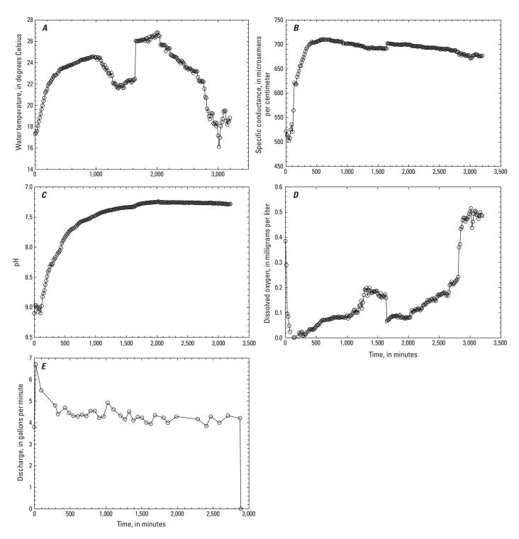
**Figure 20.** Graphs showing water temperature (*A*), specific conductance (*B*), pH (*C*), dissolved oxygen (*D*), and discharge (*E*) from the U.S. Geological Survey Hualapai Test Well during the 48-hour pumping test, western Hualapai Plateau, Arizona.
