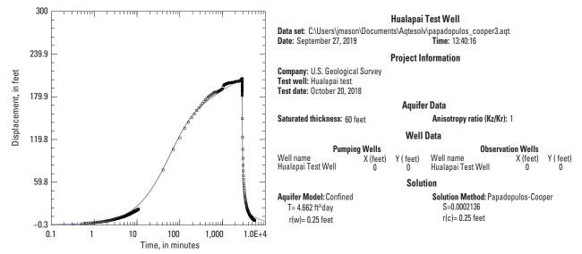
**Figure 19.** Graph and table showing estimated aquifer properties using the Papadopulos and Cooper solution for nonleaky confined aquifers for U.S. Geological Survey Hualapai Test Well on the western Hualapai Plateau, Arizona (Papadopulos and Cooper, 1967); ft²/day refers to foot squared per day.
