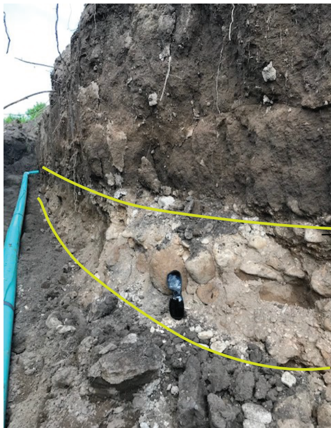
Figure 8. The inside of a trench dug in the Sun Valley Estates subdivision showing a layer of mostly cobble- and boulder-sized clasts between fine-grained clays and silts within the alluvium in north Summerset, South Dakota, with sunglasses about 5 inches in length to provide scale.
