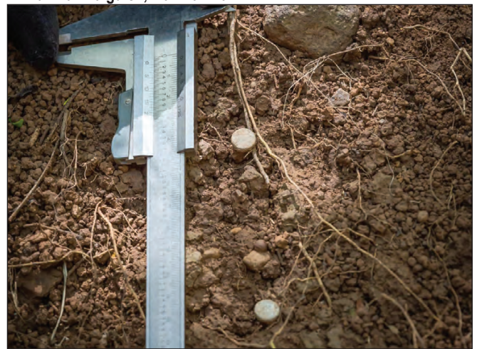
Figure 31. Bank erosion of historic fill terraces, West Maui. A, Pāpua 1 detail; B, Pāpua 2 detail; C, Honolua; D, Māhinahina detail. Exposed nails and roots show surface lowering by bank erosion over approximately 1 year of observation (15-centimeter-long calipers for scale).
