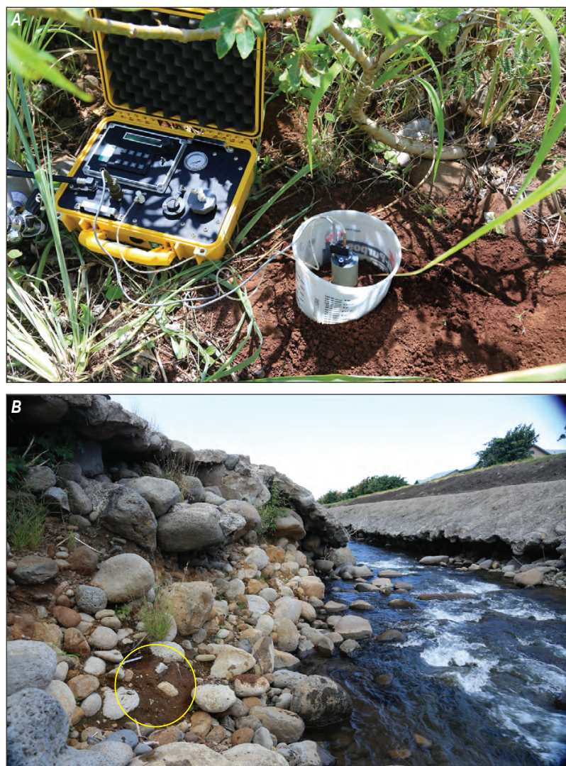
Figure 14. Illustration of Partrac's cohesive strength meter (CSM) deployed at A, Wahikuli Gulch fill terrace and B, Ōao Stream, to characterize debris-flow-deposit matrix for a related project. A, The air tank along left edge pressurizes an internal water reservoir that the instrument pumps to a jet nozzle inside the gray cup in the bucket. During testing, both the gray test vessel and the surrounding bucket are filled with water to simulate submergence. These kinds of experiments provide estimates of how resistant fill-terrace material will be to erosion by streams. B, Test area shown by yellow circle.
