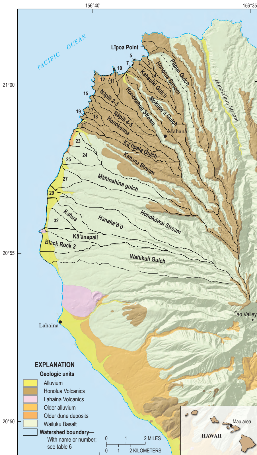
Figure 2. Map showing geology and major watersheds (unnamed watersheds are numbered) of West Maui draped over shaded-relief topography. Larger watersheds have steep headwaters characterized by rockfall and landslide processes and, towards the shore canyons, cut into low-relief surfaces composed of volcanic and alluvial deposits. A cap of bright-red-orange silts and fine sands over volcanic rock is a likely source of sediment-rich plumes polluting the nearshore after rainfalls. Geology from Sherrod and others (2007).
