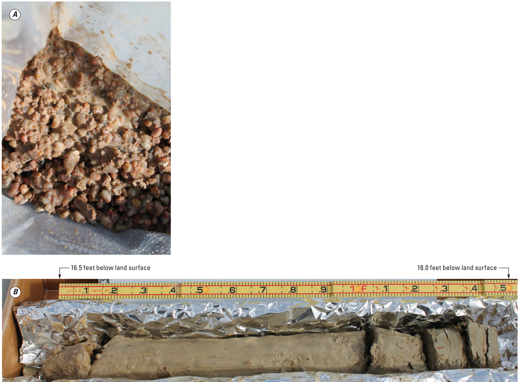
Figure 12. Cuttings and core from Quaternary older alluvial fan deposits, exploratory borehole LC-F1, southeastern Laramie County, Wyoming. A , cuttings from 29.5 feet below land surface (ft BLS) showing muddy sandy gravel; B , lateral view of core from 16.5 to 18.0 ft BLS showing muddy sand.
