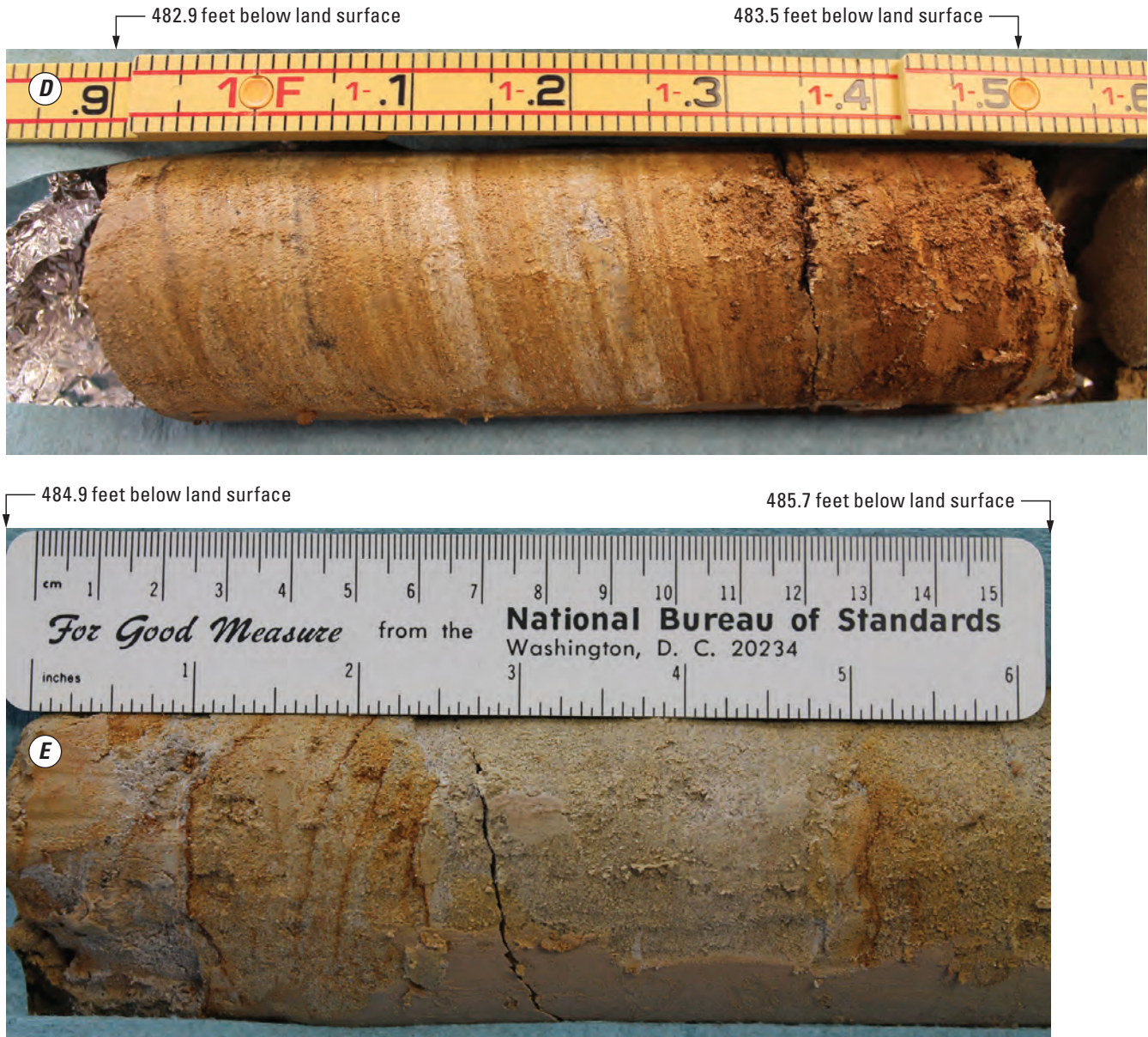
Figure 18. Core and various characteristics of parts of the Lance Formation muddy sandstone (470.1–488.1 feet below land surface [ft BLS]) in which monitoring well LN–1 was completed, exploratory borehole LC–F1, southeastern Laramie County, Wyoming. A , lateral view of core from 472.0 to 473.9 ft BLS showing muddy sandstone. Colors and color banding shown in this photograph and photographs of underlying depth intervals in this sandstone bed (fig. 18 B–E ) are common to other sandstone beds in the “lighter-colored” part of the Lance Formation; B , close-up lateral view of core from 473.25 to 473.85 ft BLS showing part of muddy sandstone interval shown in figure 18 A . Surface of core has been carefully scraped to reveal sedimentary characteristics that were not easily seen in figure 18 A ; C , lateral view of core from 482.9 to 484.7 ft BLS showing lateral view of muddy sandstone bed; D , close-up lateral view of core from 482.9 to 483.5 ft BLS showing part of muddy sandstone interval shown in figure 18 C . Surface of core has been carefully scraped to reveal sedimentary characteristics that were not easily seen in figure 18 C ; E , close-up lateral view of core from 484.9 to 485.7 ft BLS showing muddy sandstone. Surface of core has been carefully scraped to reveal sedimentary characteristics.—Continued
