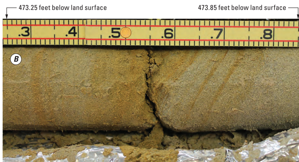
Figure 18. Core and various characteristics of parts of the Lance Formation muddy sandstone (470.1–488.1 feet below land surface [ft BLS]) in which monitoring well LN–1 was completed, exploratory borehole LC–F1, southeastern Laramie County, Wyoming. A , lateral view of core from 472.0 to 473.9 ft BLS showing muddy sandstone. Colors and color banding shown in this photograph and photographs of underlying depth intervals in this sandstone bed (fig. 18 B–E ) are common to other sandstone beds in the “lighter-colored” part of the Lance Formation; B , close-up lateral view of core from 473.25 to 473.85 ft BLS showing part of muddy sandstone interval shown in figure 18 A . Surface of core has been carefully scraped to reveal sedimentary characteristics that were not easily seen in figure 18 A ; C , lateral view of core from 482.9 to 484.7 ft BLS showing lateral view of muddy sandstone bed; D , close-up lateral view of core from 482.9 to 483.5 ft BLS showing part of muddy sandstone interval shown in figure 18 C . Surface of core has been carefully scraped to reveal sedimentary characteristics that were not easily seen in figure 18 C ; E , close-up lateral view of core from 484.9 to 485.7 ft BLS showing muddy sandstone. Surface of core has been carefully scraped to reveal sedimentary characteristics.
