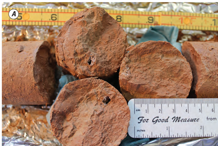
Figure 13. Core and various characteristics of the White River Formation, exploratory borehole LC-F1, southeastern Laramie County, Wyoming. A , core from 55.6 to 56 feet below land surface (ft BLS) showing voids in sandy mudstone; B , lateral view of core from 304.2 to 306.1 ft BLS showing sparse greenish-gray mottling in moderate yellowish-brown mudstone and claystone; C , lateral view of core from 344.4 to 346.3 ft BLS showing greenish-gray mottling in moderate yellowish-brown mudstone and claystone; D , lateral view of core from 394.6 to 396.5 ft BLS showing greenish-gray mottling in moderate yellowish-brown mudstone and claystone. Note brown coloration on parts of greenish-gray core is drilling mud, not sediment color. Greenish-gray mottling is more prevalent in this depth interval than in overlying depth intervals (fig. 13 C, D ); E , view perpendicular to core at 121 ft BLS showing part of muddy sandstone open to the well screen of monitoring well BR-1.
