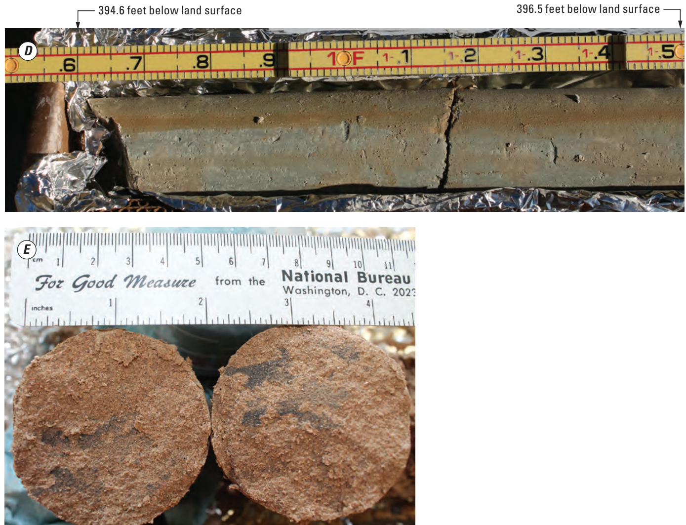
Figure 13. Core and various characteristics of the White River Formation, exploratory borehole LC-F1, southeastern Laramie County, Wyoming. A , core from 55.6 to 56 feet below land surface (ft BLS) showing voids in sandy mudstone; B , lateral view of core from 304.2 to 306.1 ft BLS showing sparse greenish-gray mottling in moderate yellowish-brown mudstone and claystone; C , lateral view of core from 344.4 to 346.3 ft BLS showing greenish-gray mottling in moderate yellowish-brown mudstone and claystone; D , lateral view of core from 394.6 to 396.5 ft BLS showing greenish-gray mottling in moderate yellowish-brown mudstone and claystone. Note brown coloration on parts of greenish-gray core is drilling mud, not sediment color. Greenish-gray mottling is more prevalent in this depth interval than in overlying depth intervals (fig. 13 C , D ); E , view perpendicular to core at 121 ft BLS showing part of muddy sandstone open to the well screen of monitoring well BR-1.—Continued
