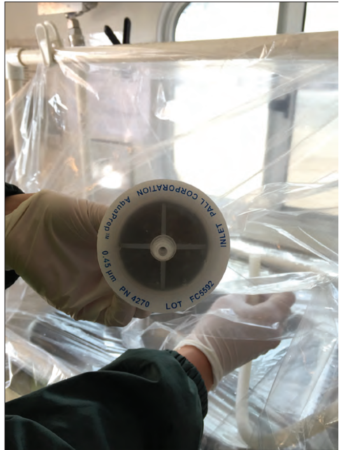
Figure 12. A, Samplers retrieved from VA-1A that have black precipitate on the outsides, and B, filter from VA-1A, where black precipitate formed in the processing filter. Photographs by Alanna Jornigan, U.S. Geological Survey.
