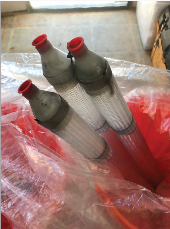
Figure 12. A, Samplers retrieved from VA-1A that have black precipitate on the outsides, and B, filter from VA-1A, where black precipitate formed in the processing filter. Photographs by Alanna Jornigan, U.S. Geological Survey.
