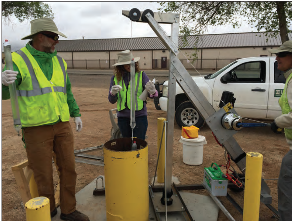
Figure 4. Dual-membrane passive diffusion bag sampler retrieval at Veteran’s Administration well site, Kirtland Air Force Base, Albuquerque, New Mexico.
