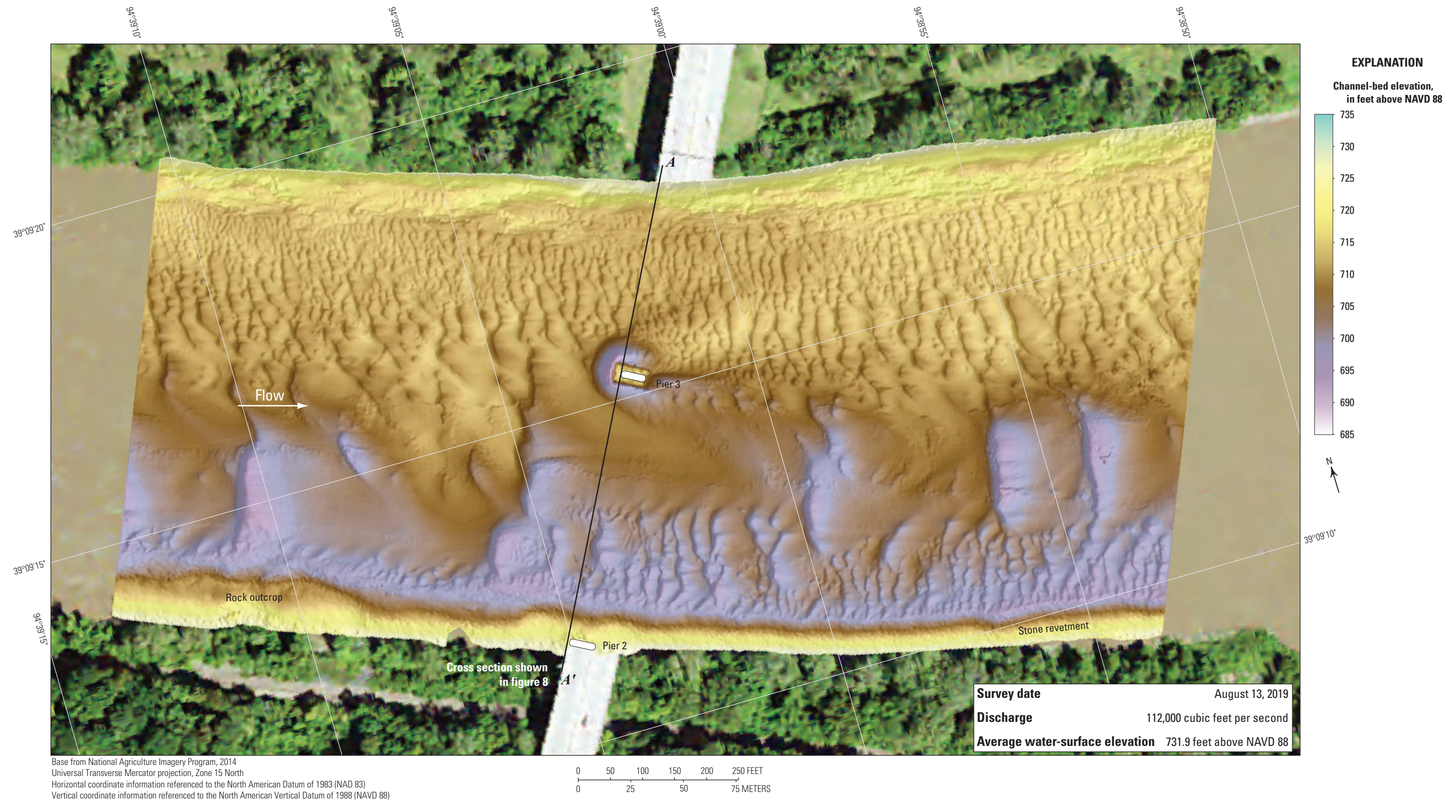
Figure 6. Bathymetric survey of the Missouri River channel near structure A1800 on Interstate 635 in Kansas City, Missouri, on August 13, 2019.
