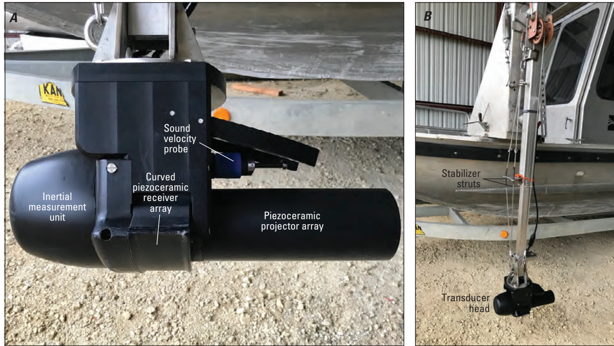
Figure 3. The Norbit iWBMSH multibeam echosounder. Photographs by Richard J. Huizinga, U.S. Geological Survey. A , Viewed from the side. B , Mounted on the port side of the U.S. Geological Survey boat.
