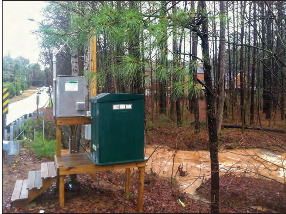
Figure 2. Multiparameter stream monitoring site, Little Stone Mountain Creek, DeKalb County, Georgia, August 2017 (U.S. Geological Survey site number 02207135). Photograph by Andrew E. Knaak, U.S. Geological Survey.
