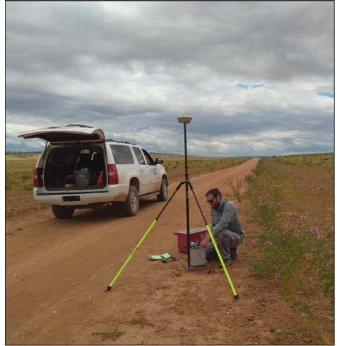
Figure 7. Photograph of relative gravity meter (Zero-Length Spring, Inc., Burris relative-gravity meter B44) and Global Positioning System (GPS) rover setup at an observation point for the gravity transects during this study. The study area is in Coconino Plateau, Coconino County, Arizona. U.S. Geological Survey photograph taken by Libby Wildermuth in 2019.
