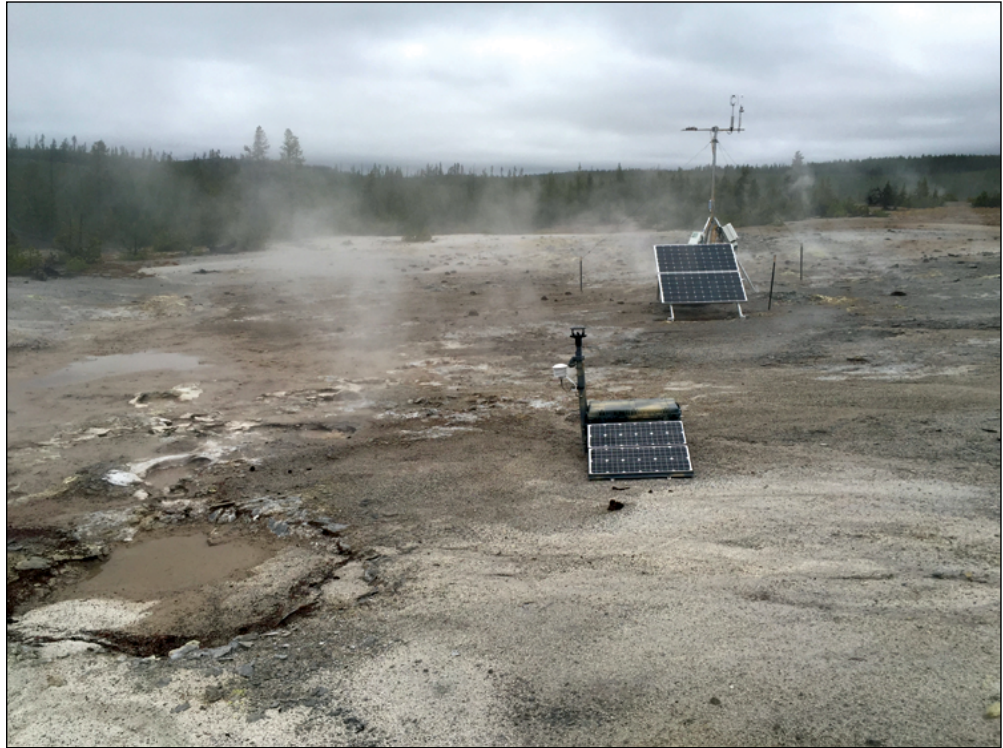
Figure 9. Photograph showing a continuous gas-monitoring station deployed near Norris Geyser Basin. The station in the foreground is a Multi-GAS instrument, and behind it is an eddy covariance station. U.S. Geological Survey photograph by Jen Lewicki on October 3, 2016. Research conducted under Yellowstone Research Permit YELL-2016-SCI-7082.
