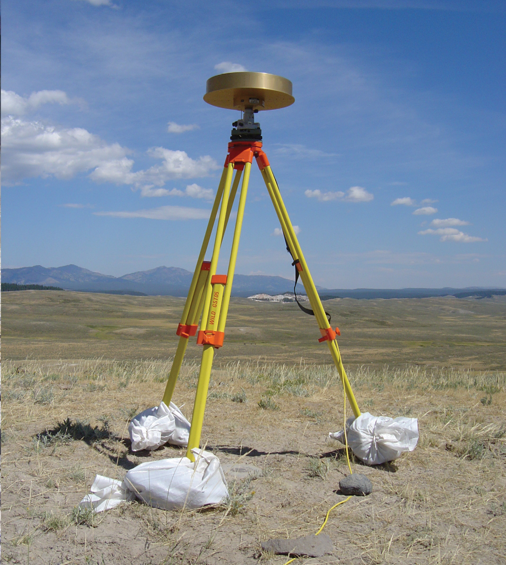
Photograph of campaign GPS station in Hayden Valley, Yellowstone National Park. GPS monitoring was conducted under permit YELL-2003-SCI-0114. Photograph taken by Jamie Farrell, University of Utah, August 13, 2003.
