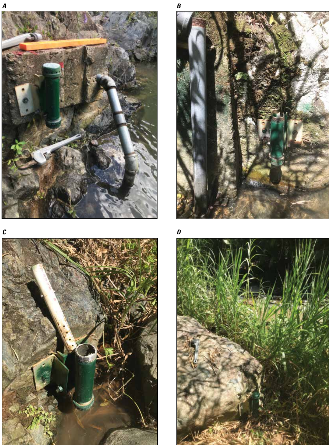
Figure 4.3. Pressure transducers installed at A , CSA1, B , CSA2, C , CSA3, and D , CSA4 at station 50093000 Río Marín near Patillas. Date of photographs is October 21, 2020. Photographs by Manuel Rosario, U.S. Geological Survey.
