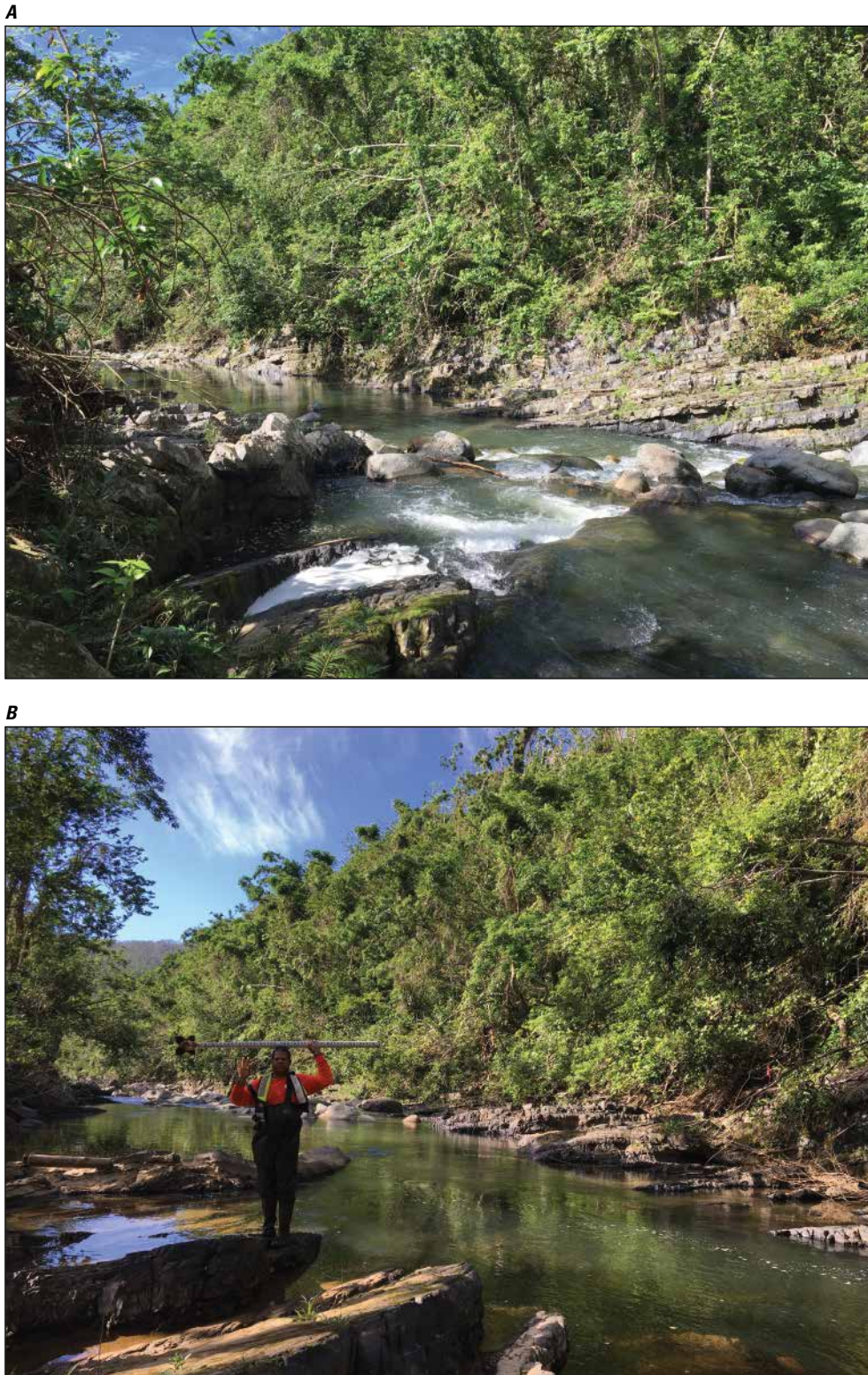
Figure 2.9. Conditions along study reach for station 50065500 Río Mameyes near Sabana, November 27, 2017. A , View downstream at middle part of study reach; B , view downstream at lower part of study reach; rod held at approximate high-water-mark level for the peak streamflow of October 15, 2017. Photographs by Julieta Gómez-Fragoso, U.S. Geological Survey.
