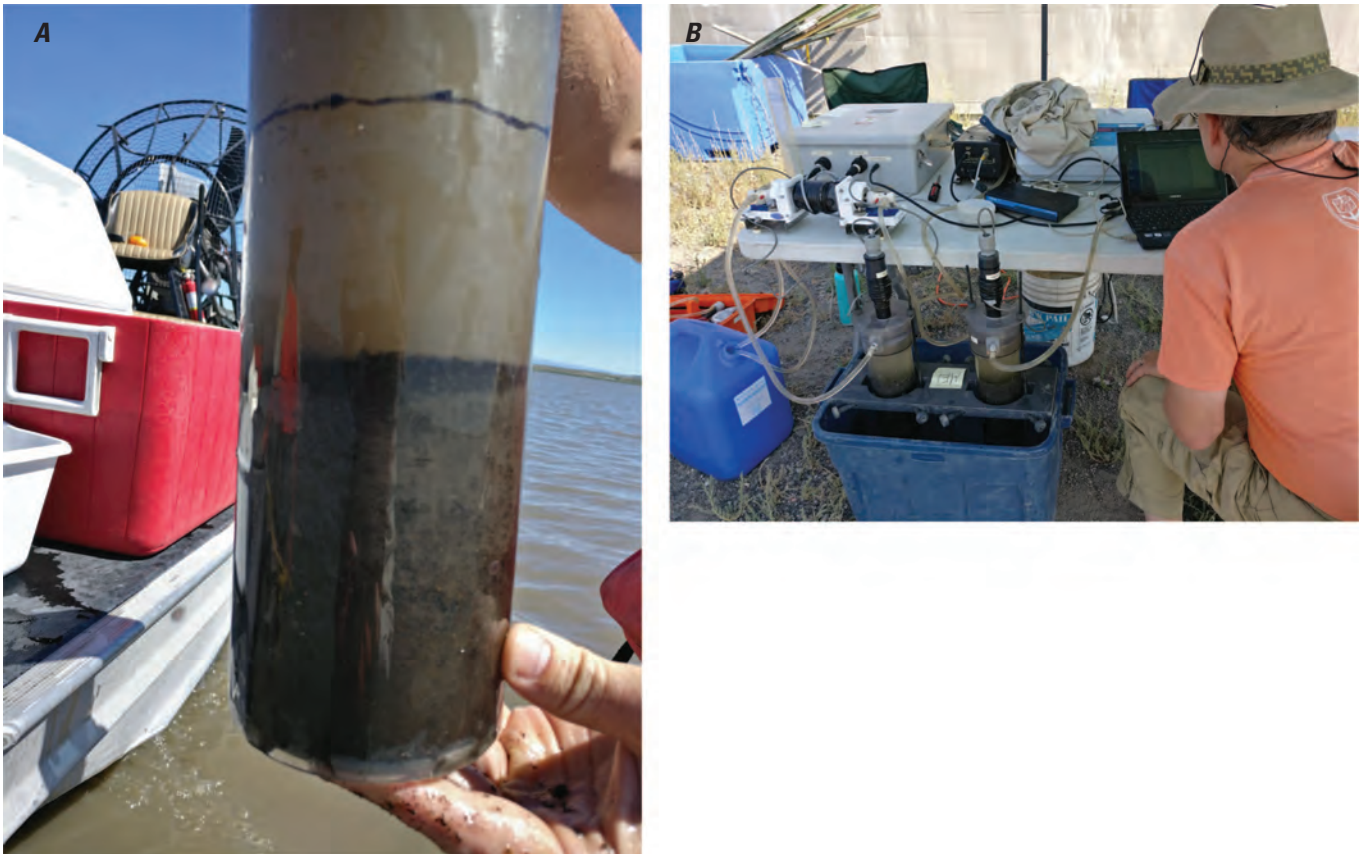
Figure 4.2. Photographs showing (A) one of the sediment lake cores collected in August 2018 and (B) the mobile erosion laboratory setup on land, at Malheur Lake, Oregon. Photographs by Joe Barnett, U.S. Fish and Wildlife Service.
