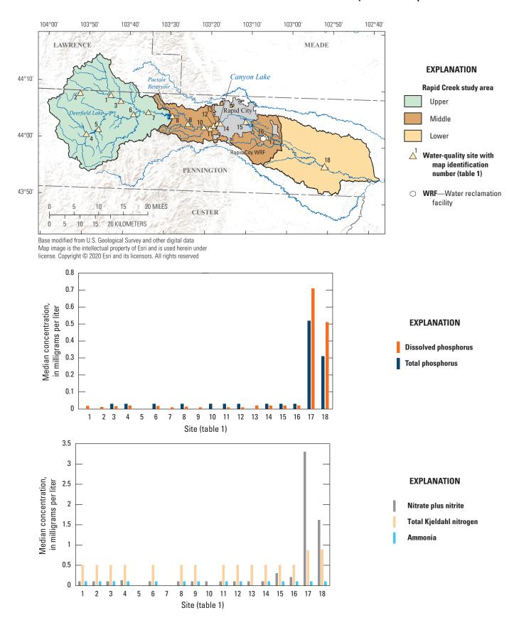
**Figure 5.** Median concentrations of nitrate plus nitrite, total Kjeldahl nitrogen, ammonia, dissolved phosphorus, and total phosphorus in the Rapid Creek Basin. Sites are ordered from upstream to downstream by site number (table 1).
