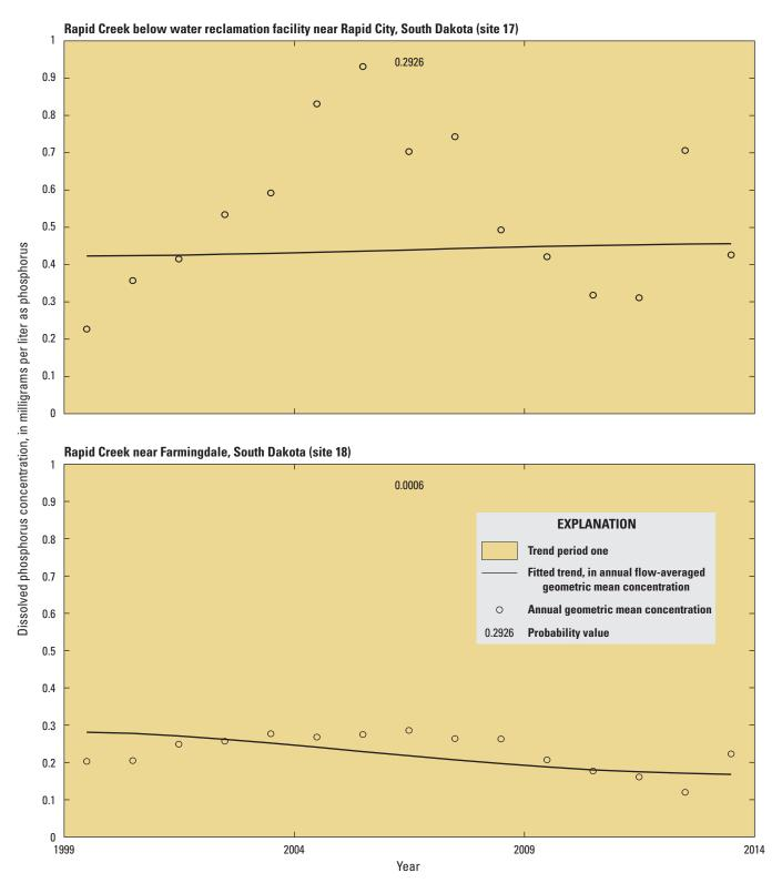
**Figure 20.** Fitted trends for dissolved phosphorus in annual flow-averaged geometric mean concentration of dissolved phosphorus at two sites with annual geometric mean concentrations in the Rapid Creek Basin for the trend period (1999–2014).
