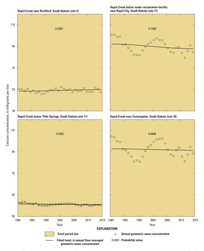
**Figure 10.** Fitted trends for calcium in annual flow-averaged geometric mean concentration of calcium at four sites in the Rapid Creek Basin for the trend period (1989–2019).
