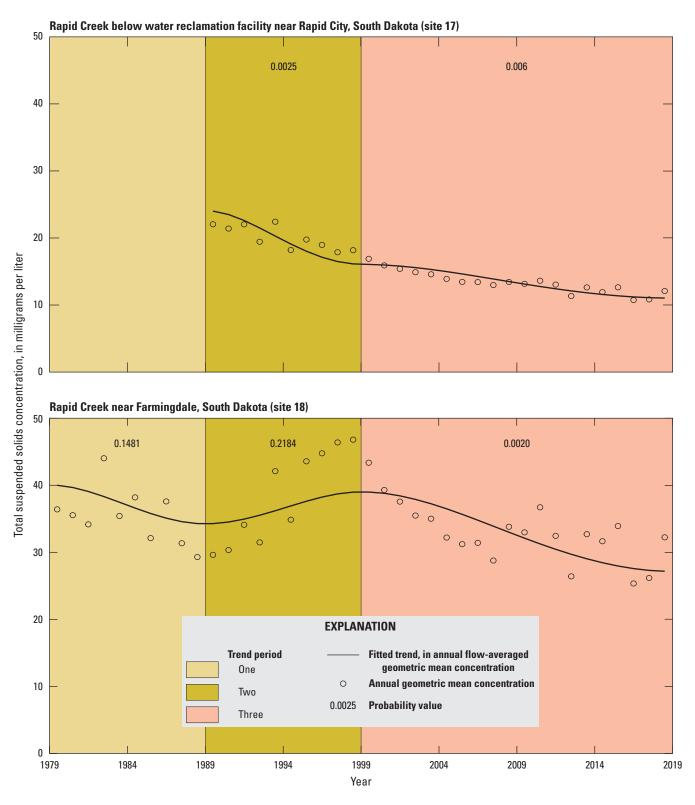
**Figure 16.** Fitted trends for total suspended solids in annual flow-averaged geometric mean concentration of total suspended solids at two sites with annual geometric mean concentrations in the Rapid Creek Basin for the trend period (1979–2019).
