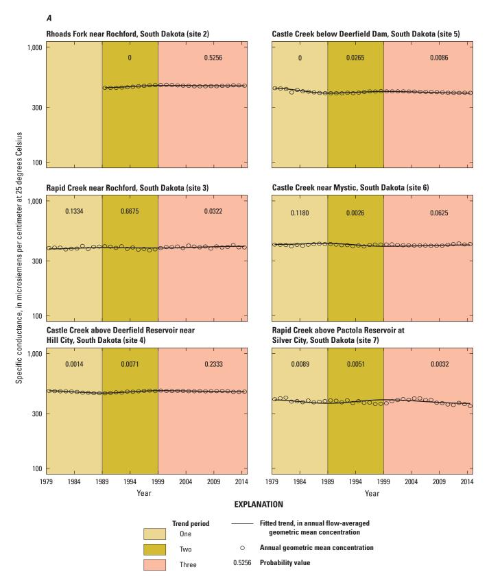
**Figure 14.** Fitted trends for specific conductance in annual flow-averaged geometric mean concentration of specific conductance at 12 sites with annual geometric mean concentrations for specific conductance in the Rapid Creek Basin for the trend period (1979–2014). *A*, upper basin; *B*, middle and lower basin.
