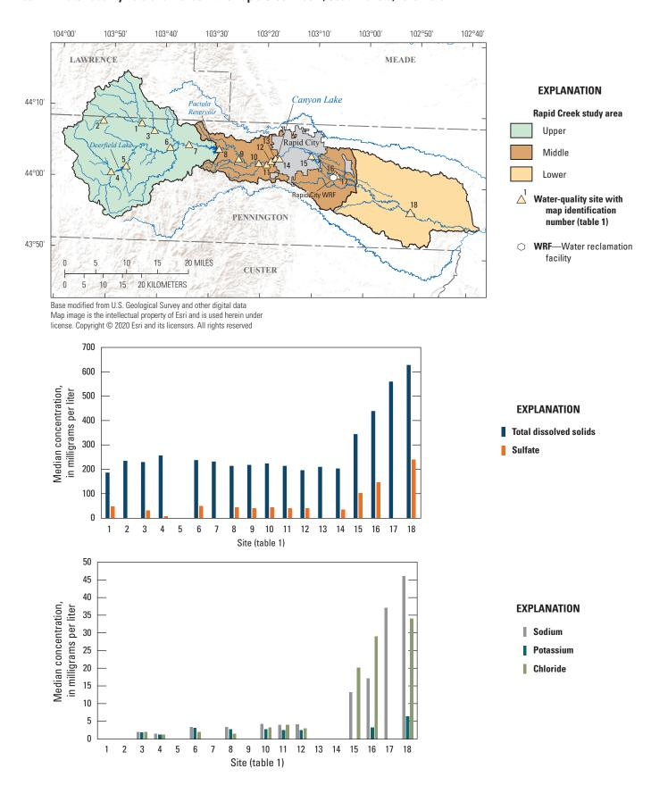
Figure 3. Median concentrations of total dissolved solids, sulfate, sodium, potassium, and chloride in the Rapid Creek Basin. Sites are ordered from upstream to downstream by site number (table 1).
