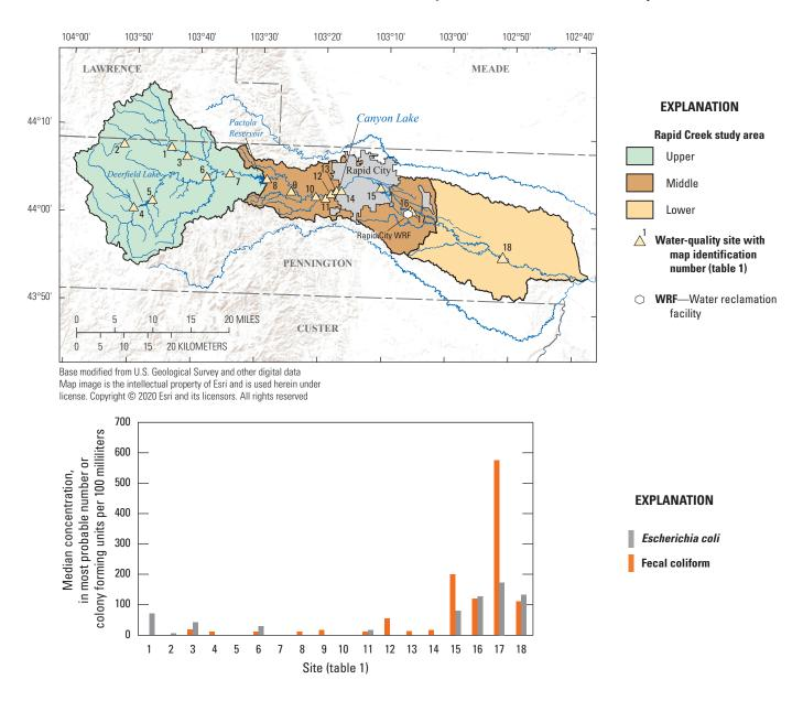
**Figure 7.** Median concentrations of *Escherichia coli* (in most probable number per 100 milliliters) and fecal coliform concentrations (in colony forming units per 100 milliliters) in the Rapid Creek Basin. Sites are ordered from upstream to downstream by site number (table 1).
