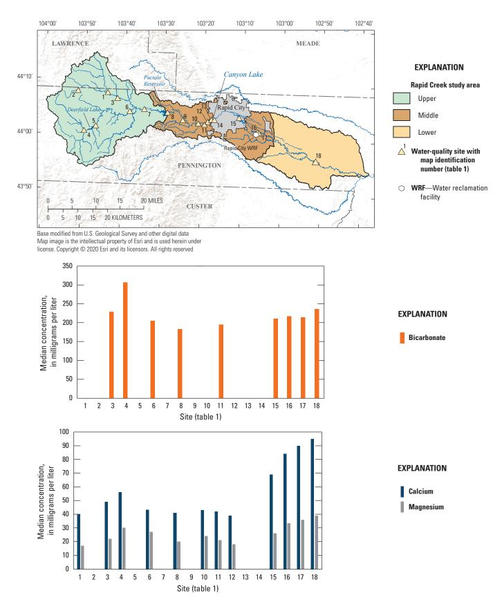
Figure 4. Median concentrations of bicarbonate, calcium, and magnesium in the Rapid Creek Basin. Sites are ordered from upstream to downstream by site number (table 1).
