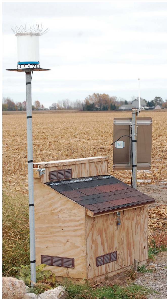
Figure 5. Equipment enclosure and rain gage at the runoff site (U.S. Geological Survey station number 041572269), in the surface-water study area, Tuscola County, Michigan; photograph by Julia Prokopec, U.S. Geological Survey.
