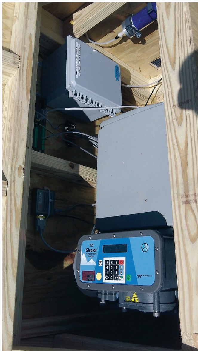
Figure 4. Composite automatic sampler and associated equipment at the Tile 17 site (U.S. Geological Survey station number 041572264), in the surface-water study area, Tuscola County, Michigan; photograph by Carol Luukkonen, U.S. Geological Survey.
