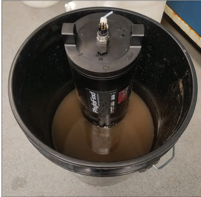
Figure 8. Photograph showing a Turner Designs, Inc. PhytoFind in-place phytoplankton classification tool in the test vessel in a solution of soil and a mixed-population phytoplankton culture for turbidity testing; photograph by the U.S. Geological Survey.
