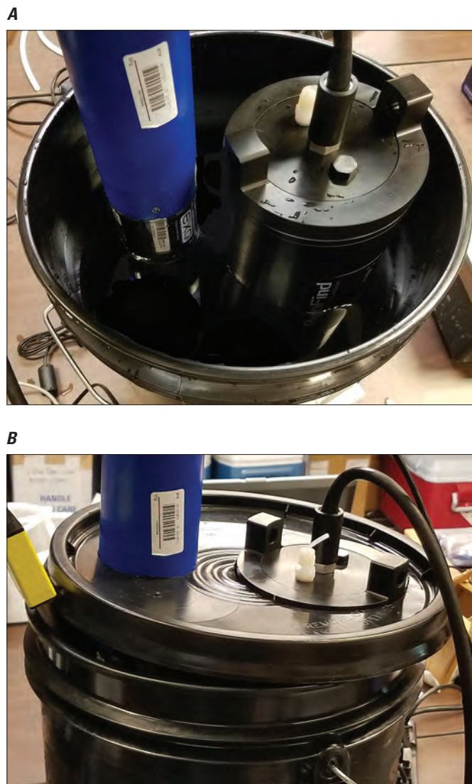
Figure 3. Photographs showing configuration of the Turner Designs, Inc. PhytoFind in-place phytoplankton classification tool and YSI Inc. EXO Total Algae-PC sensor mounted on a YSI, Inc. EXO2 multiparameter sonde for laboratory testing. View A , underneath the test vessel lid and B , with test vessel lid in place, as used during testing. Photographs by the U.S. Geological Survey.
