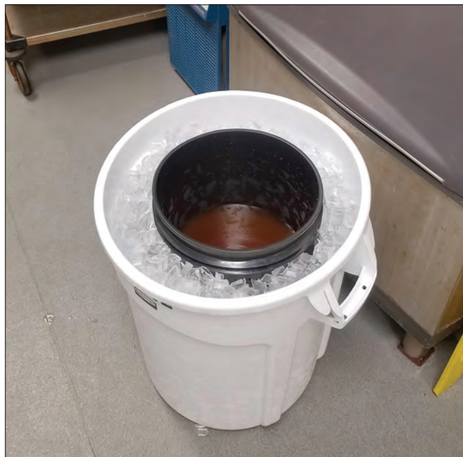
Figure 5. Photograph showing a solution of rhodamine water tracer and basic blue 3 dyes, chilling in the test vessel by submersion in ice and rock salt; photograph by the U.S. Geological Survey.
