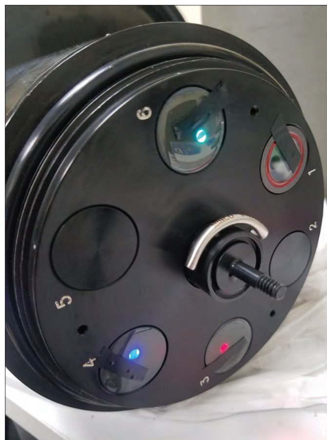
Figure 4. Photograph showing small strips of black electrical tape covering the photodetectors of the Turner Designs, Inc. PhytoFind in-place phytoplankton classification tool to prevent the detection of any light during the baseline signal test; photograph by the U.S. Geological Survey.
