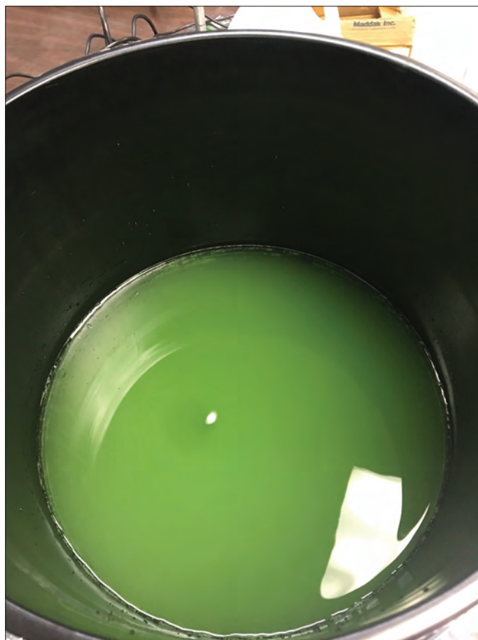
Figure 7. Photograph showing the Synechococcus culture mechanically mixing in the test vessel. The test vessel sits atop the magnetic stir plate (not pictured). Photograph by the U.S. Geological Survey.
