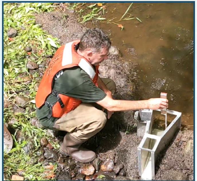
Photograph of a low streamflow measurement made using a Parshall flume at the Pendleton Hill Brook near Clarks Falls, Connecticut (0118300) U.S. Geological Survey streamgage on August 11, 2022; photograph from video by Nigel Pepin, U.S. Geological Survey.
