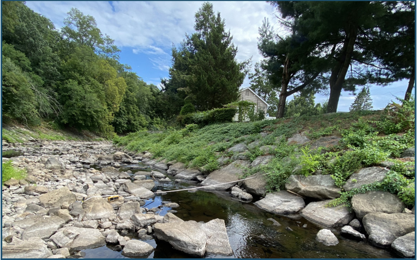
Photograph of a low flow measurement section used at the Byram River at Pemberwick, Connecticut (01212500) U.S. Geological Survey streamgage on August 17, 2022; photograph by Maria Skarzynski, U.S. Geological Survey.
