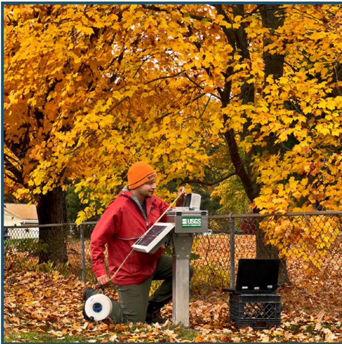
Photograph of a groundwater level measurement taken at the MA–HHW 1R Hardwick, Mass. (422058072085101) U.S. Geological Survey real-time monitoring well in Hardwick, Massachusetts, on October 17, 2022; photograph by Samuel Banas, U.S. Geological Survey.
