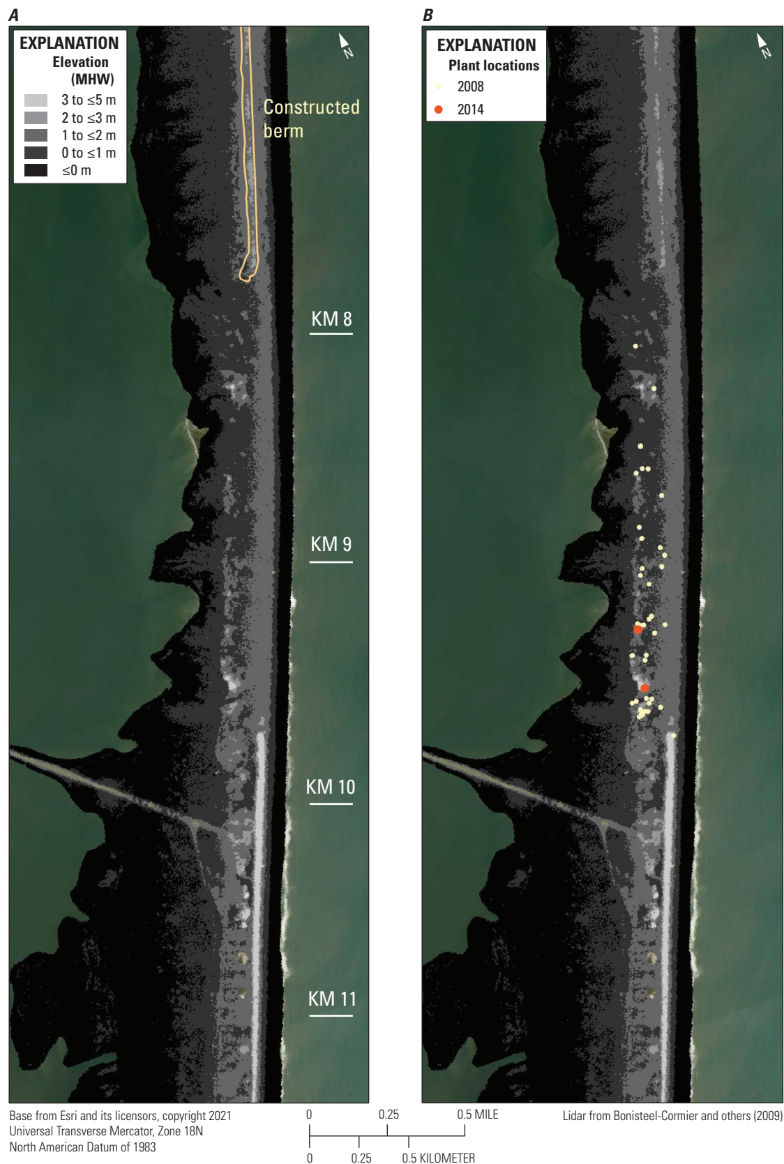
Figure 19. Light detection and ranging (lidar) elevation maps of northern Assateague Island between kilometer markers (KMs) 7 and 11. A , Map shows the footprint of a berm constructed in 1999 to reduce the possibility of overwash. B , Map shows the 2008 and 2014 observed seabeach amaranth locations. MHW, mean high water; m, meter; <, less than.
