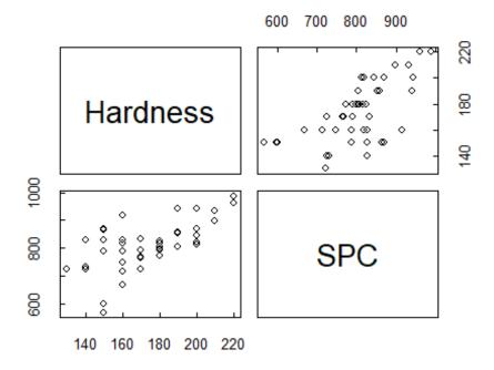
The x- and y-axis labels for a given bivariate plot are defined by the intersecting row and column labels.
