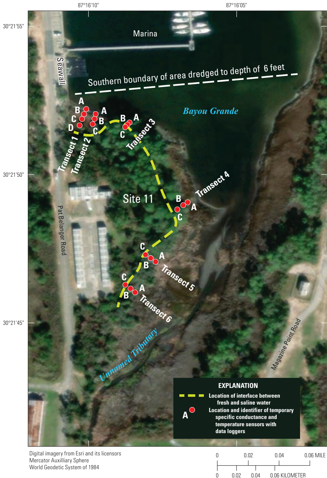
Figure 26. Approximate horizontal location of the fresh groundwater/saline surface-water interface at low tide, Site 11 and Bayou Grande, Naval Air Station Pensacola, during the study period based on documentation of visible seeps, infrared camera surveys, the fiber-optic distributed temperature sensing survey, and continuous water temperature and specific conductance data collected from the data loggers at the six transects.
