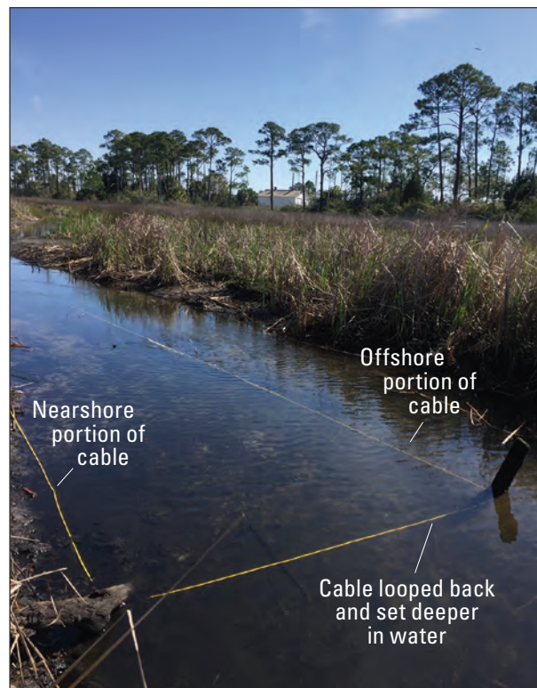
Figure 18. A, Three-night mean water temperatures, from 4:00 p.m. to 4:00 a.m. central daylight time the following day, along the fiber-optic cable, for the March 13–16 fiber-optic distributed temperature sensing survey. In this plot, the cable is deployed in surface water at 207 meters (m; nearshore cable portion), looped at 575 m, as shown in B, and returns back as the offshore cable portion, remaining underwater until placed overland at 227 m. Groundwater temperature is roughly 15.5 °C. Values below that temperature indicate very shallow and cooler surface water covering the cable or the subaerial exposure of the cable to cooler night air, especially to the extreme left, where the outer cable was placed over land.
