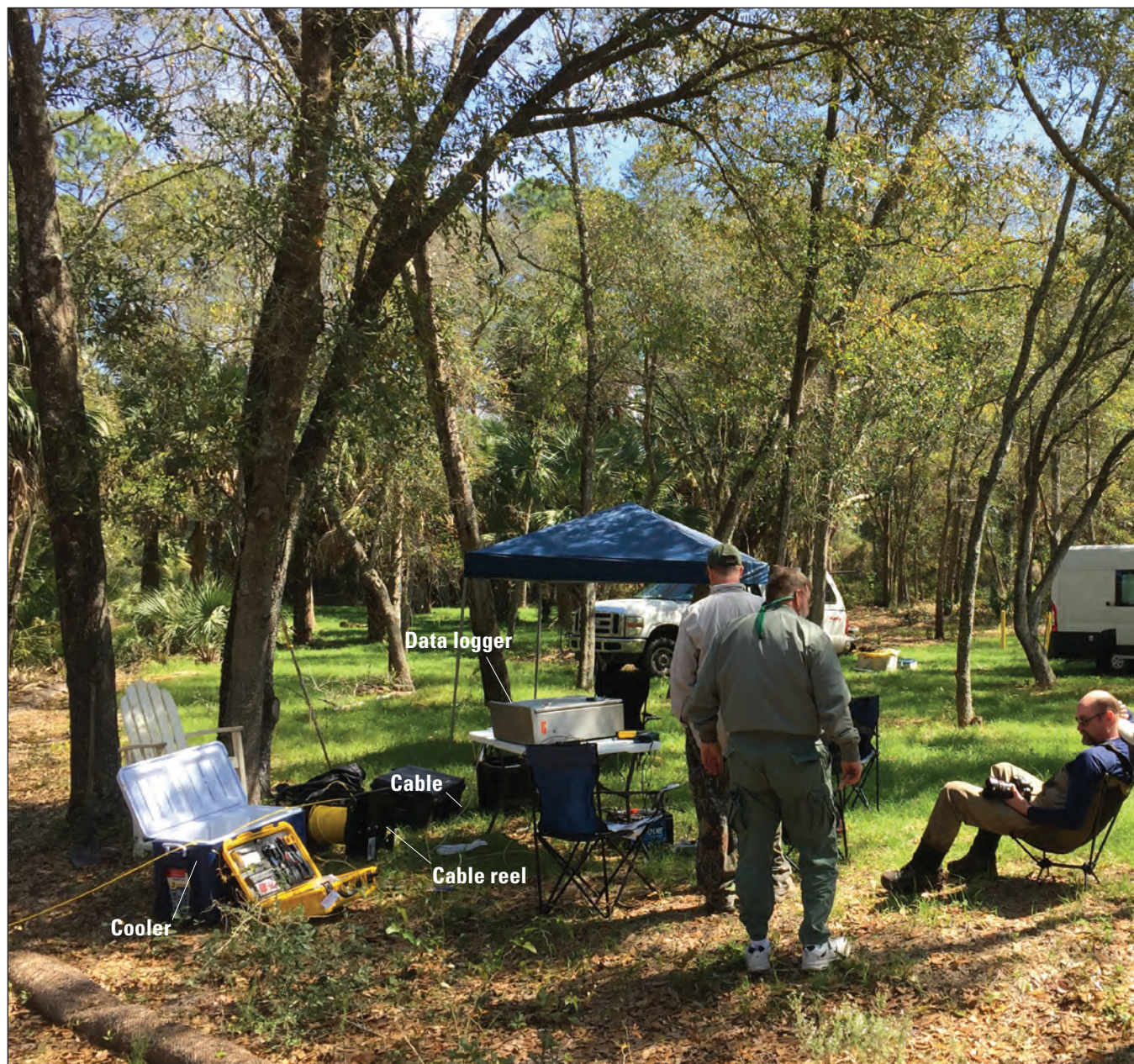
Figure 10. The offshore cable path near the end running through a cooler filled with ice (left) to the data logger on the table (center). The area shown is a densely vegetated upland part of Site 11.
