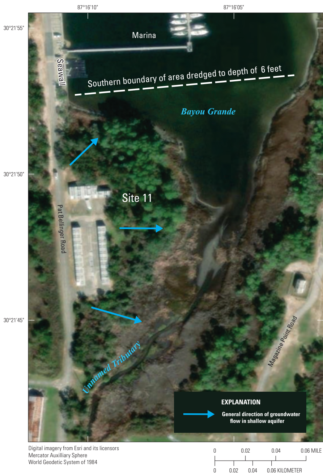
Figure 3. Study area of Site 11 described in this report and Bayou Grande, Naval Air Station Pensacola, and generalized direction of groundwater flow in the shallow aquifer. The greater depth of surface water north of the dredging boundary line is indicated by the darker color of surface water.
