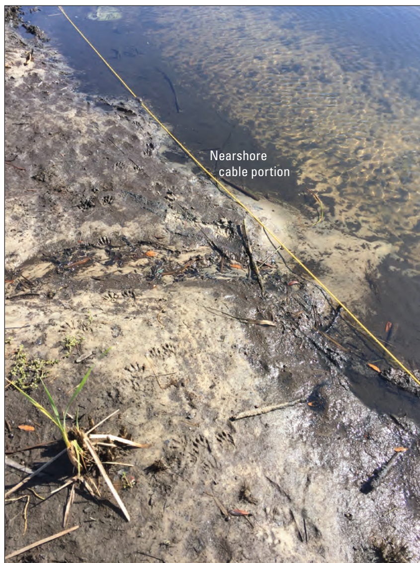
Figure 9. Location of inner (nearshore) portion of the fiber-optic cable and flow entering surface water from a seep located inland during low tide at Bayou Grande.
