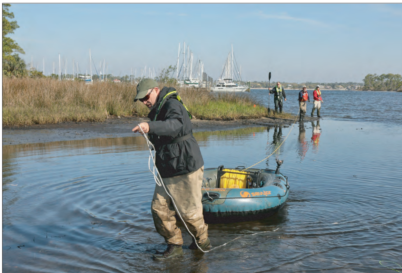
Figure 7. The unspooling of the fiber-optic cable from the raft in Bayou Grande.
