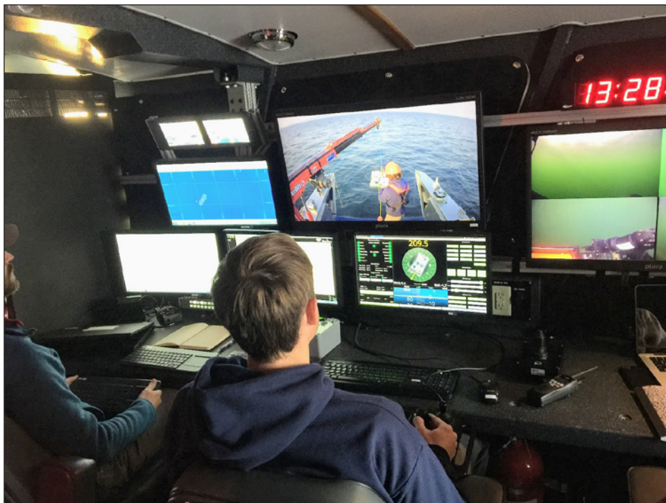
Figure F2. Photograph showing scientists aboard research vessel (RV) Annie II monitoring control room video of the remotely operated vehicle (ROV) Yogi being deployed in Yellowstone Lake, Wyoming, August 2017. The ROV made heat-flow measurements at a thermal field on the lake floor as part of the multiyear Hydrothermal Dynamics of Yellowstone Lake (HD-YLAKE) project (Sohn and others, 2017). Photograph by S. Hurwitz, U.S. Geological Survey.
