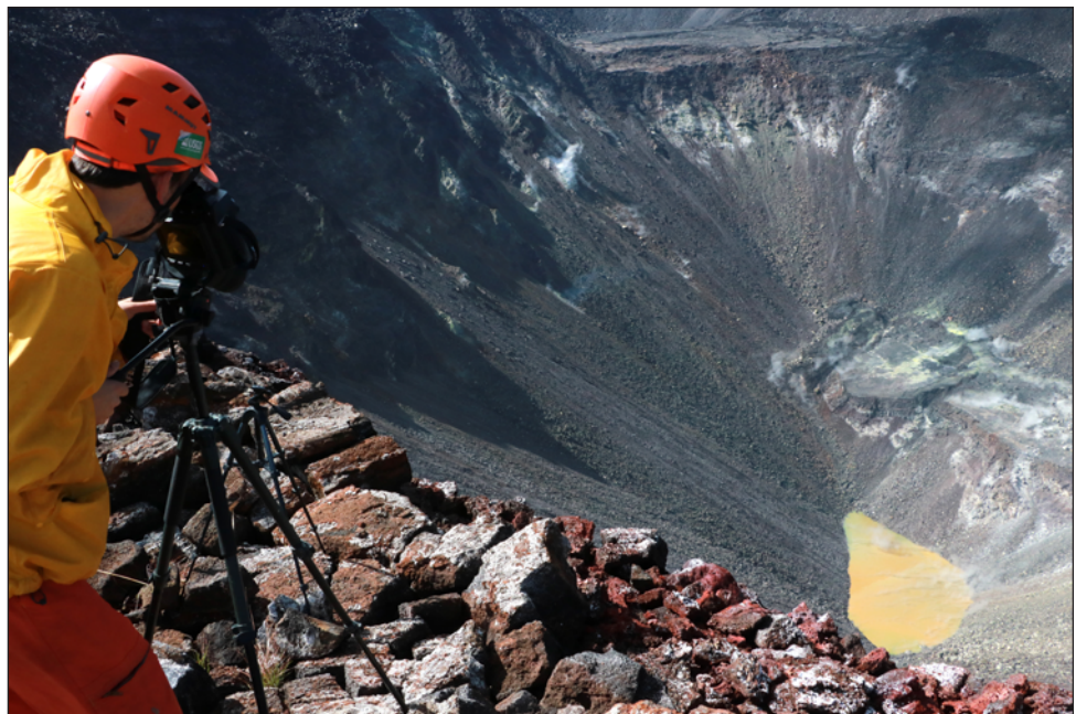
Figure F1. Photograph showing U.S. Geological Survey Hawaiian Volcano Observatory geologist measuring lake-surface temperatures using a thermal camera at Kīlauea's short-lived crater lake. Flat areas of lava flow surfaces beyond and above the lake are former sections of the crater floor of Halema'uma'u that subsided hundreds of meters during the 2018 caldera collapse. Yellow areas are regions of substantial sulfur precipitation. Photograph by K. Mulliken, U.S. Geological Survey, December 18, 2019.
