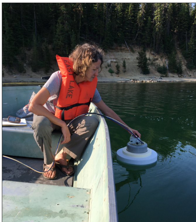
Figure F3. Photograph showing U.S. Geological Survey California Volcano Observatory geologist measuring CO 2 flux on the surface of East Lake, Newberry Crater, Oregon. Photograph by L. Clor, U.S. Geological Survey, July 29, 2020.
