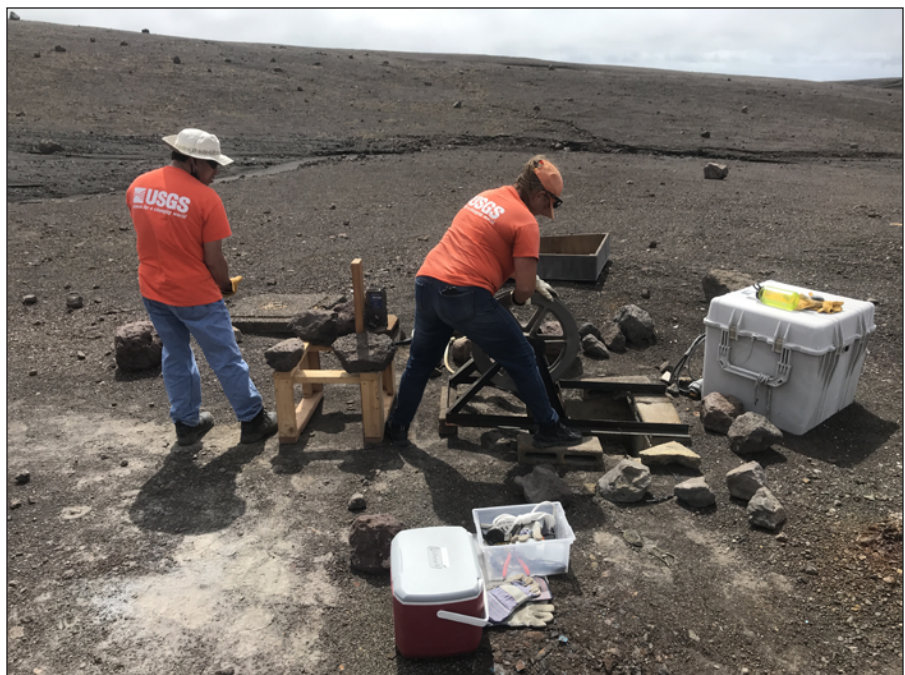
Figure K1. Photograph showing U.S. Geological Survey Hawaiian Volcano Observatory staff measuring water-table depth and collecting water samples for analysis from the 1,262-meter-deep NSF Well in the summit caldera of Kīlauea, Hawai‘i. Photograph by F. Younger, U.S. Geological Survey, March 22, 2022.
