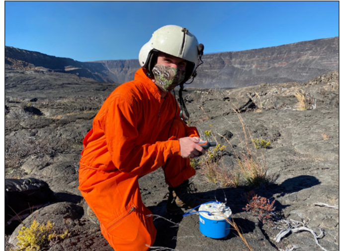
Figure M1. Photograph showing U.S. Geological Survey Hawaiian Volcano Observatory geophysicist P. Dotray deploying a 5-second geophone in Halema'uma'u as part of a rapid response to the December 20, 2020, eruption of Kīlauea, Hawai'i. These instruments were made available through the Incorporated Research Institutions for Seismology (IRIS) Portable Array Seismic Studies of the Continental Lithosphere (PASSCAL) Instrument Center. Photograph by J. Chang, U.S. Geological Survey, January 3, 2021.
