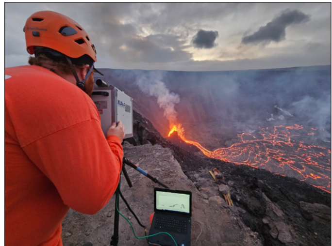
Figure M2. Photograph showing U.S. Geological Survey Hawaiian Volcano Observatory gas scientist M. Cappos using a field-portable Fourier-transform infrared (FTIR) spectrometer on the rim of Halema'uma'u to measure gas composition during the June 7, 2023, eruption of Kīlauea, Hawai'i. The FTIR measures the composition of emitted gases by measuring how the volcanic plume absorbs infrared energy. The plume generated by the summit eruption was sulfur-dioxide (SO 2 ) rich, but also contained water vapor, carbon dioxide, and halogen gases, such as HCl and HF. Photograph by P. Nadeau, U.S. Geological Survey, June 7, 2023.
