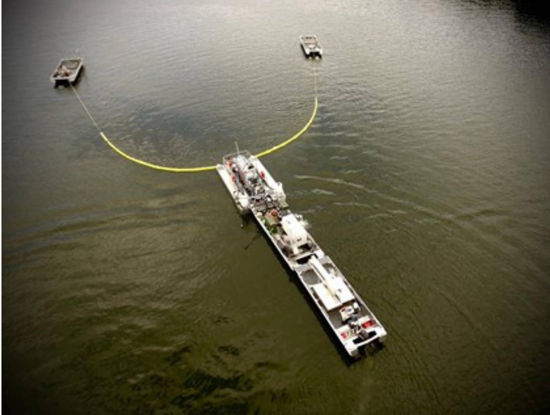
Figure 4. Aerial photograph of an interesting alternative-format shipboard HABITATS prototype being tested in Chautauqua Lake, New York, in September 2020. As described by Page and others (2021, p. 23), the “shipboard interception system consisted of two lead boats with two 50 ft [50-foot] tow booms connected to a floating weir skimmer intake on the front of a trailing DAF [dissolved air flotation] barge.” HABITATS, Harmful Algal Bloom Interception, Treatment, and Transformation System. Photograph courtesy of John Kennedy, New York State Department of Environmental Conservation; used with permission. It was also used in Page and others (2021, fig. 2–8).
