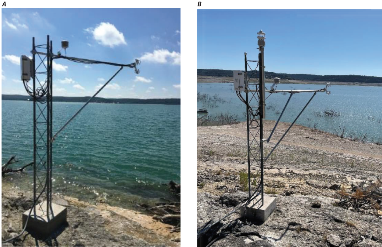
Figure 3. Photographs in A , June 2017 and B , October 2022 of the Medina Lake meteorological station, where eddy covariance evaporation data were collected on the shore of Medina Lake (U.S. Geological Survey station 293355098560601 Medina Lake meteorological station near Riomedina, Texas) (site 6) (fig. 1; table 1). Photographs by Richard Slattery, U.S. Geological Survey.
