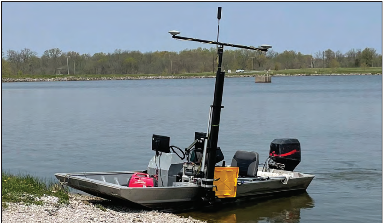
Figure 9. The multibeam echosounder. A , Viewed from the side. B , Mounted on the port side of the U.S. Geological Survey 24-foot cabin boat. C , Deployed on the port side of the 16-foot jon boat.
