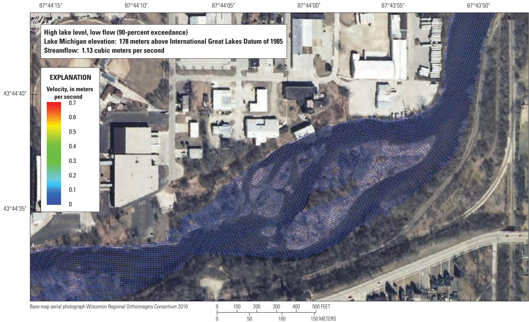
Figure 15. Velocity vectors near the Wildwood Islands complex for high Lake Michigan water levels varying Sheboygan River flows. A , Low flow. B , Medium flood. C , Large flood.
