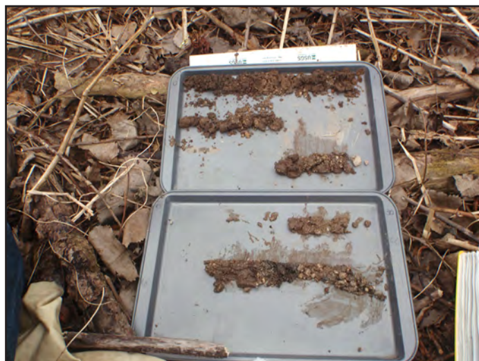
Figure 12. Photographs of gravel found on Sheboygan River bars and in cores from the Wildwood Islands complex. A , Gravel substrate on the bar near core 14.5–3. B , Gravel in core 14.5–1 with similar size to channel bar gravel of about 1.5 centimeters. Core increments on tins represent consecutive 0.3-meter increments, starting with 0 (surface) at the upper left.
