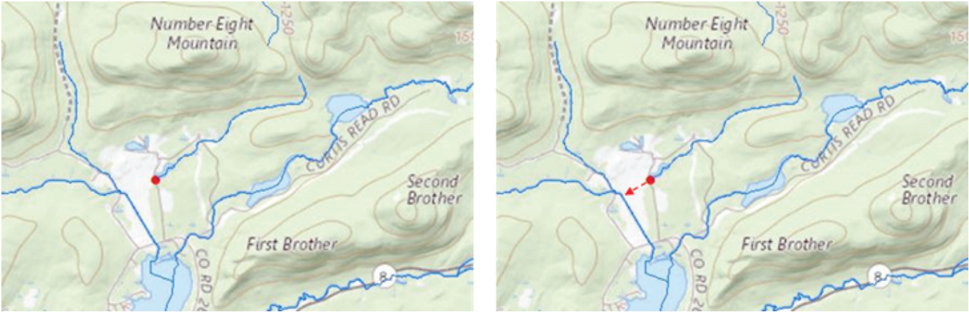
Figure 4. An example map demonstrating an ongoing effort (as of 2024) to use “nongeometric connections” to repair the network connectivity in the National Hydrography Dataset Plus High Resolution (NHDPlus HR). The red dot is the end of an isolated network that should be connected. Nongeometric connections allow tabular connections from the downstream end of an isolated network to either the upstream or downstream end of the flowline into which the flow of the water can be modeled within the NHDPlus HR network.
