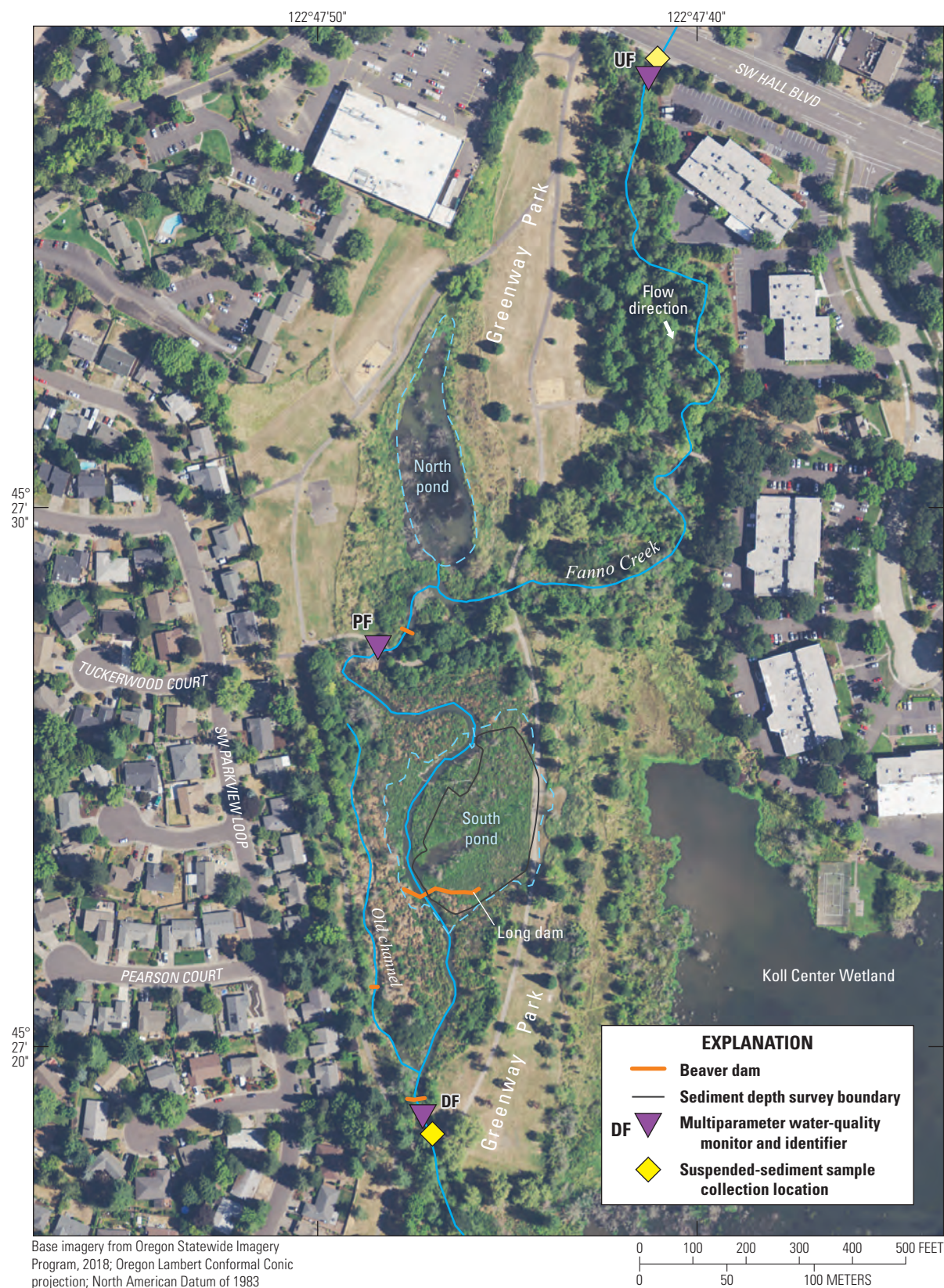
Figure 2. Fanno Creek study area, suspended-sediment sample collection locations, known beaver dams, and locations where continuous multiparameter water-quality monitors were deployed at the monitoring sites: Upstream at Fanno Creek (UF), Ponded at Fanno Creek (PF), and Downstream at Fanno Creek (DF). Additional site information is available in table 1 .
