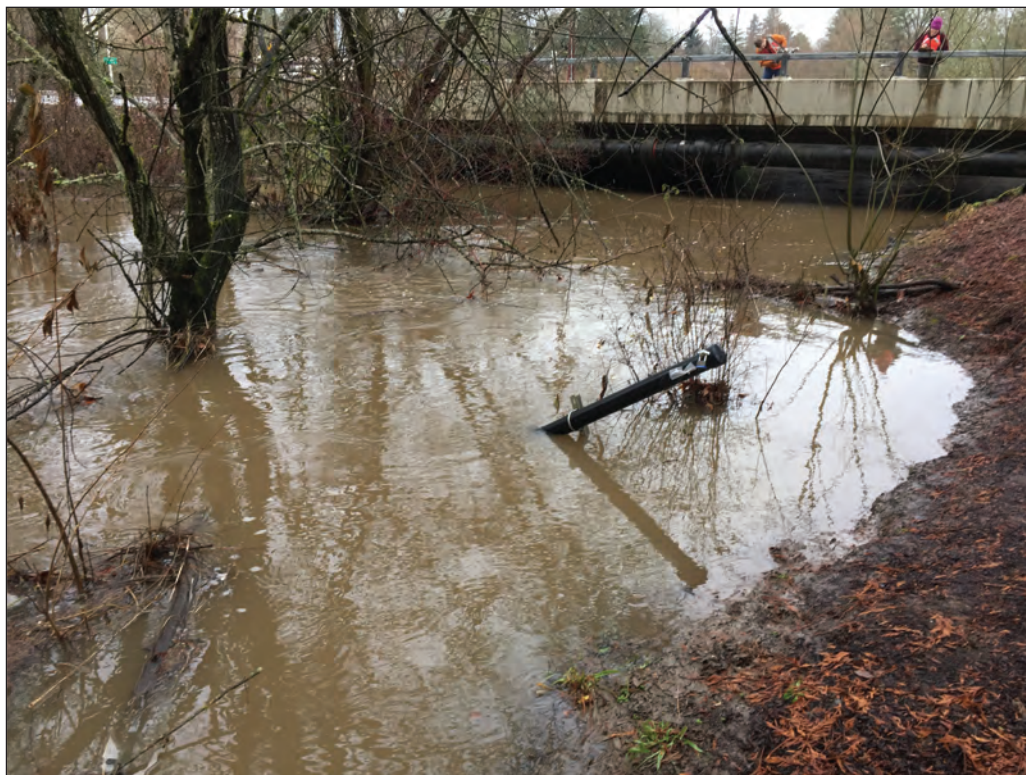
Figure 4. Water-quality monitor deployed at Fanno Creek at Greenway Park, Southwest Hall Boulevard (Upstream at Fanno Creek site) during high-flow conditions, Tualatin River Basin, northwestern Oregon. Photograph taken by Erin Leahy (U.S. Geological Survey) during storm event on March 15, 2017.
