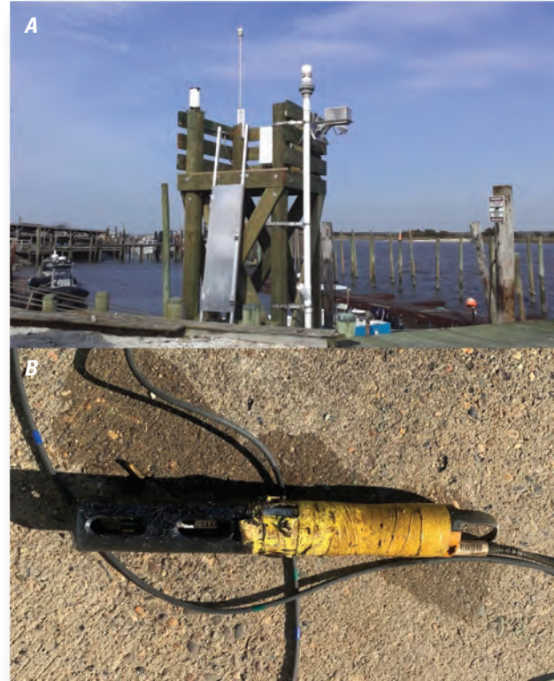
Figure 3. Photographs showing A, Maurice River at Bivalve, New Jersey (U.S. Geological Survey site no. 01412150) tide gage and B, a close-up view of a multiparameter water-quality sonde after it was removed for cleaning and calibration.
