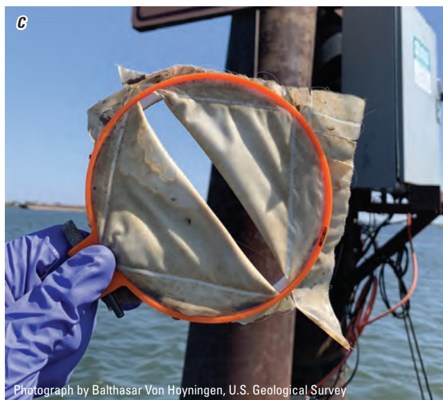
Figure 2. Examples of the different styles of Solid Phase Adsorption Toxin Tracking (SPATT) samplers: A , sachet; B , hoop; and C , combination of the sachet and hoop.
