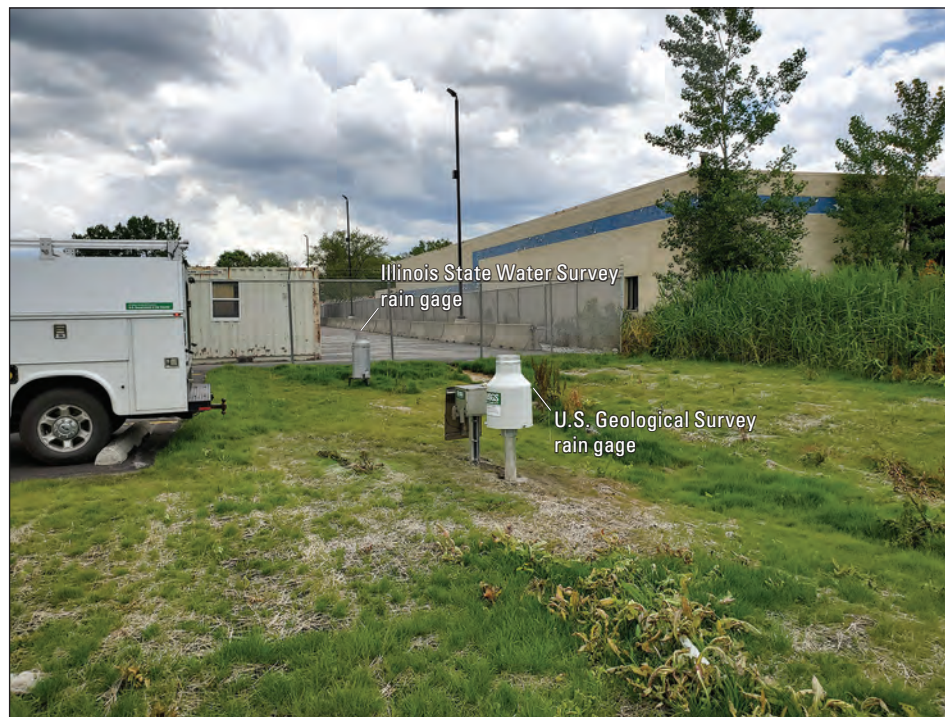
Figure 2.45. Photograph of the southwest view of the Rain Gage at Harvey, Illinois (413510087380201). Photograph by Kevin K. Johnson, U.S. Geological Survey.
