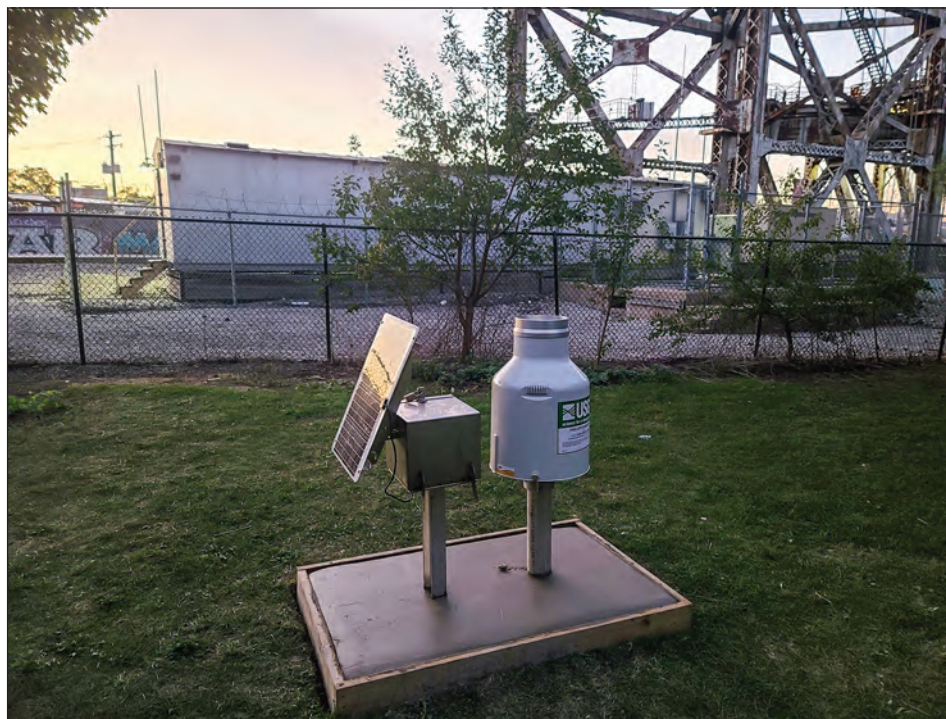
Figure 2.21. Photograph of the west view of the Rain Gage at Ping Tom Park at Chicago, Illinois (415118087381201). Photograph by Kevin K. Johnson, U.S. Geological Survey.
