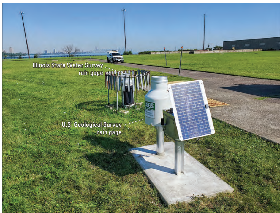
Figure 2.29. Photograph of the northeast view of the Rain Gage at South Shore, Illinois (414527087323801). Photograph by Kevin K. Johnson, U.S. Geological Survey.
