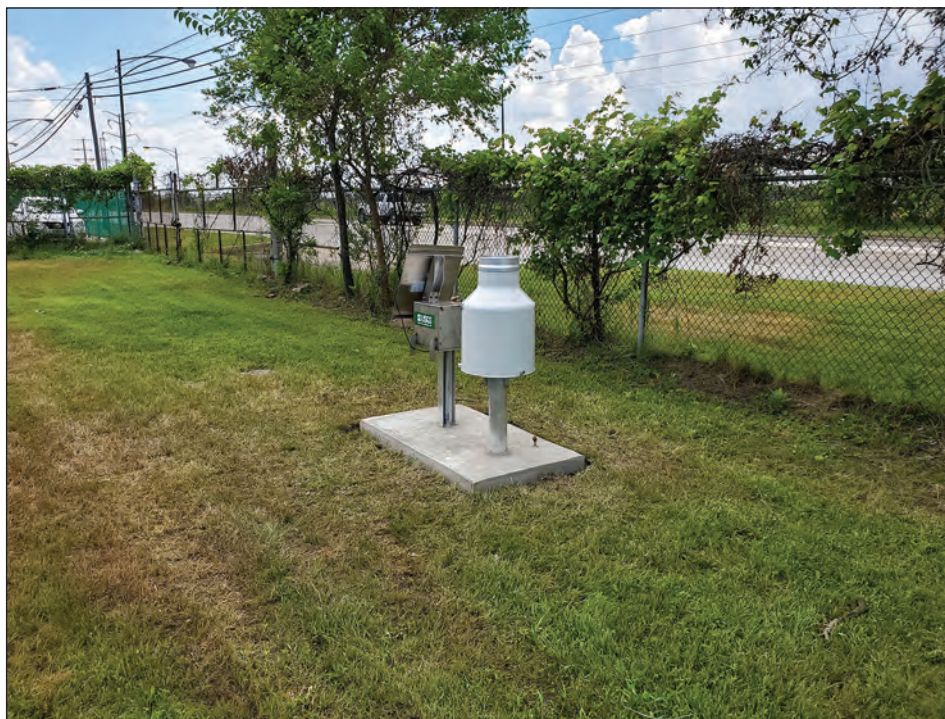
Figure 2.39. Photograph of the south view of the Rain Gage at Hegewisch, Illinois (414045087322301). Photograph by Kevin K. Johnson, U.S. Geological Survey.
