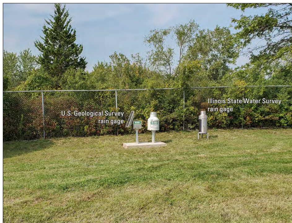
Figure 2. Photograph of the Illinois State Water Survey and U.S. Geological Survey precipitation gage installations at Rain Gage at Orland Park, Illinois (413514087523501). (Photograph by Kevin K. Johnson, U.S. Geological Survey).
