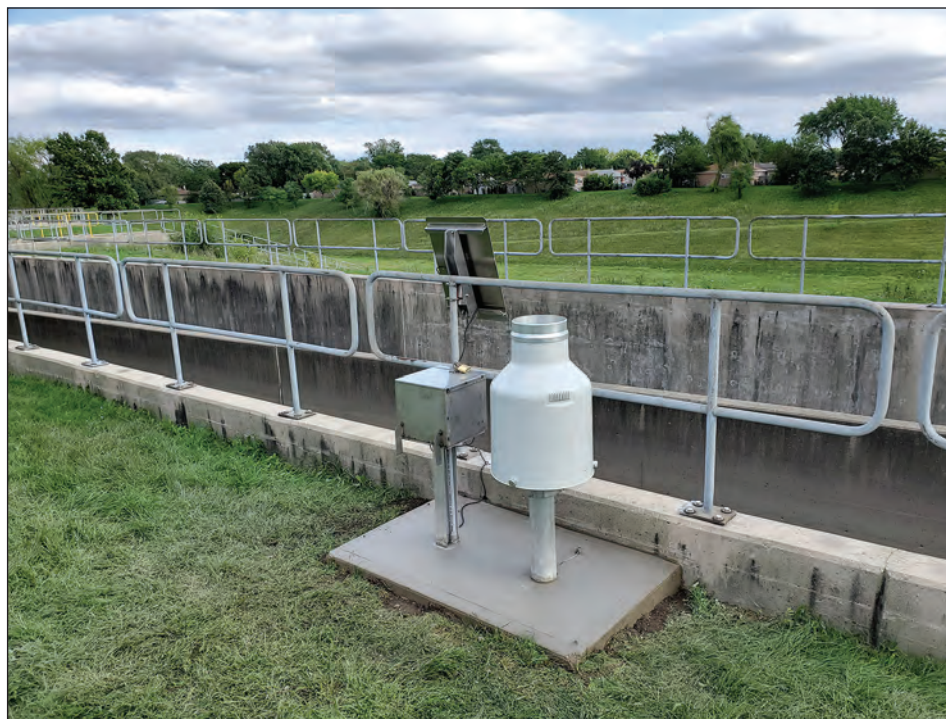
Figure 2.9. Photograph of the south view of the Rain Gage at Franklin Park, Illinois (415537087525801). Photograph by Kevin K. Johnson, U.S. Geological Survey.
