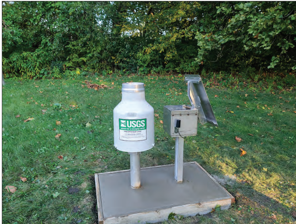
Figure 2.27. Photograph of the east view of the Rain Gage at Hamilton Park at Chicago, Illinois (414542087380901). Photograph by Kevin K. Johnson, U.S. Geological Survey.
