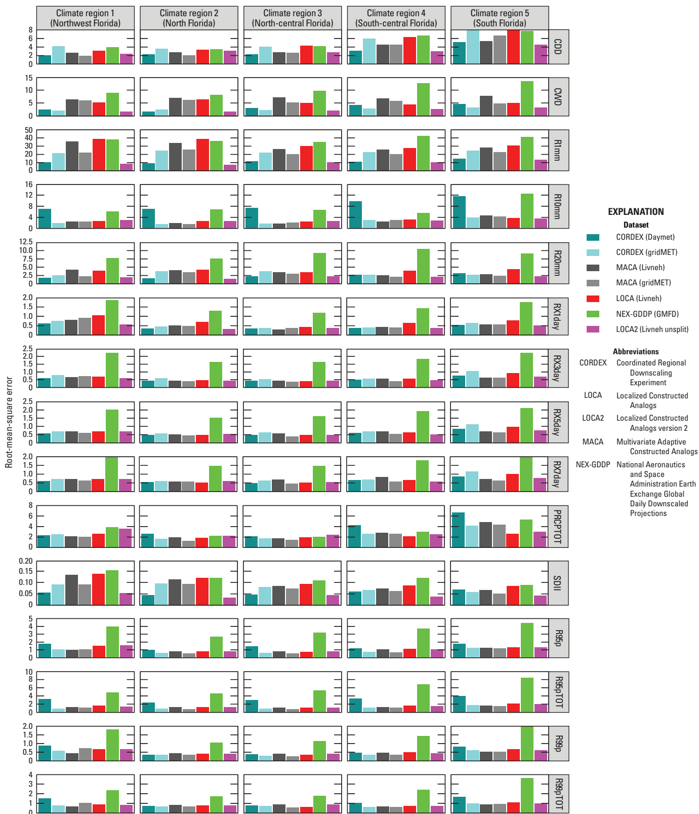
Figure 23. Median root-mean-square error (RMSE) of the climatology of extreme precipitation indices across models in each downscaled climate dataset compared against those from the Parameter-elevation Regressions on Independent Slopes Model (PRISM) for the period 1981–2005. Units for individual extreme precipitation indices are given in table 3.
