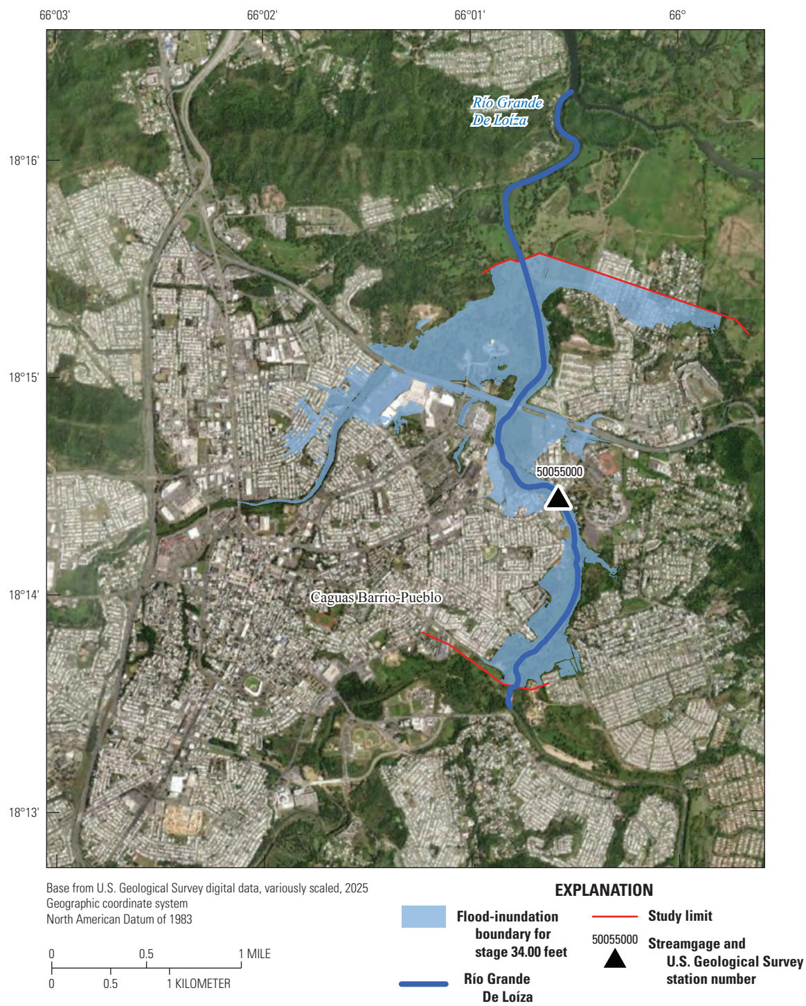
Figure 3. Map showing the floodplain boundary for stage 34.00 feet at the U.S. Geological Survey streamgage 50055000, Río Grande De Loíza at Caguas, Puerto Rico, overlain on orthorectified imagery.
