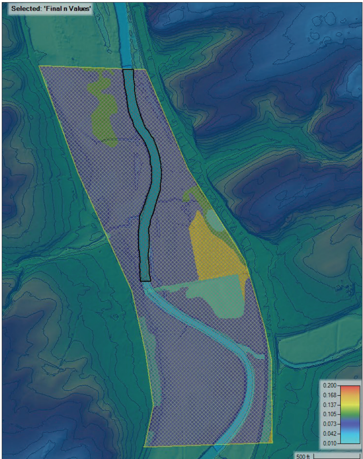
Figure 9. HEC-RAS screen capture displaying the land cover feature class and calibration region overlaid on the model terrain, demonstrating the variation in Manning's n -values around the Blackwells Mills streamgaging weir. Calibration region is outlined in black.
