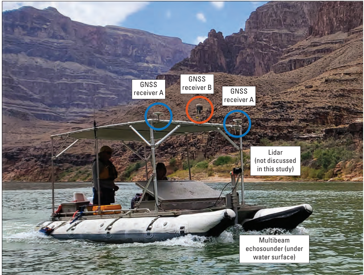
Figure 4. Photograph of the Research Vessel Frank Protiva during the study. Global navigation satellite system (GNSS) antennae for two systems were mounted to a rigid aluminum frame, which also supported a shade canopy. The multibeam echosounder was fixed to the boat with a custom mount, which allowed it to be secured above the water in rapids and deployed in pools, as shown in the photograph. lidar, light detection and ranging. Photograph by Katherine Chapman, U.S. Geological Survey.
