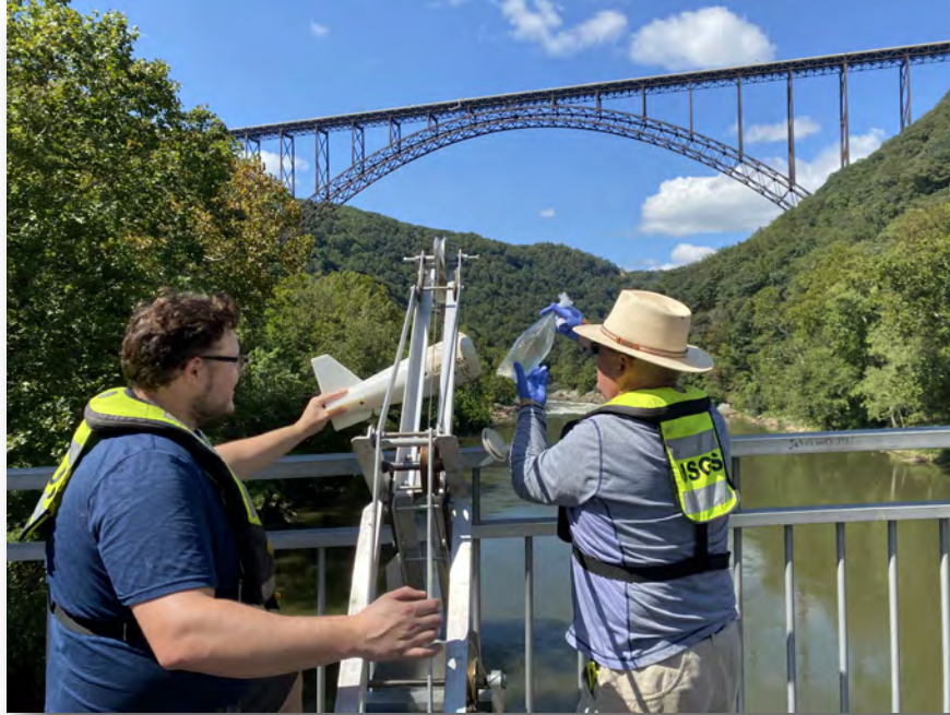
Figure 2. Photograph showing U.S. Geological Survey (USGS) personnel collecting a water sample at the Fayette monitoring location on the New River, West Virginia, in September 2022 using a DH-2 sampler and bridge crane. Photograph by Matthew R. Kearns, USGS. Additional location information is in table 1 .
