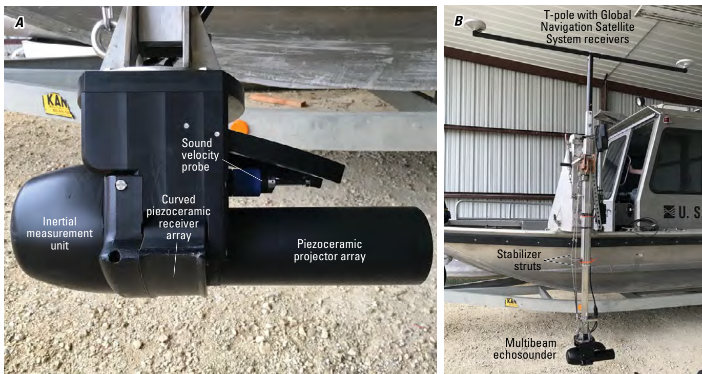
Figure 3. Photographs showing the multibeam echosounder (photographs by Richard J. Huizinga, U.S. Geological Survey). A, viewed from the side; B, viewed as mounted on the port side of the U.S. Geological Survey boat.
