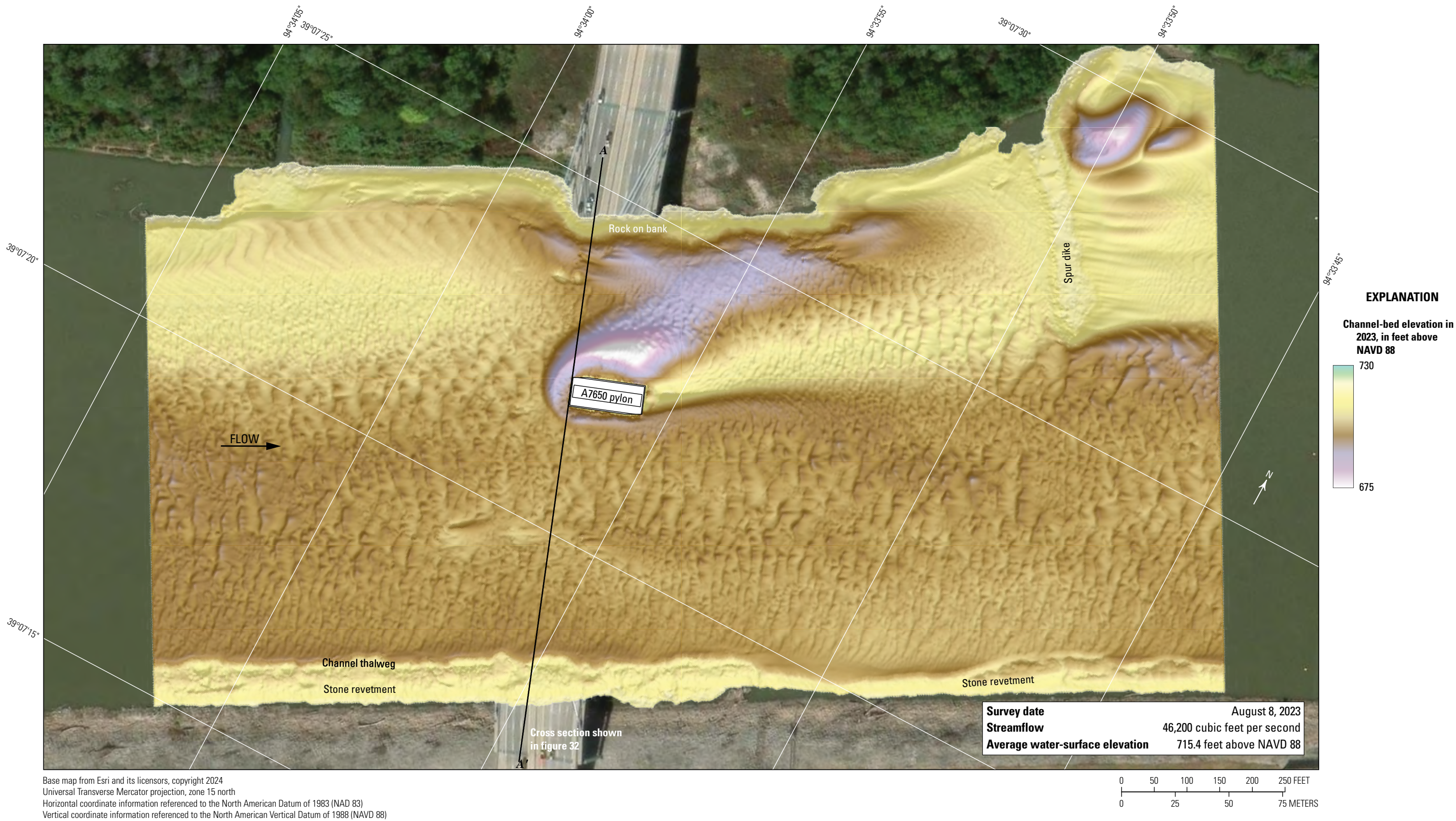
Figure 30. Map showing bathymetric survey of the Missouri River channel near structure A7650 on Interstate 35 in Kansas City, Missouri. [NAVD 88, North American Vertical Datum of 1988]
