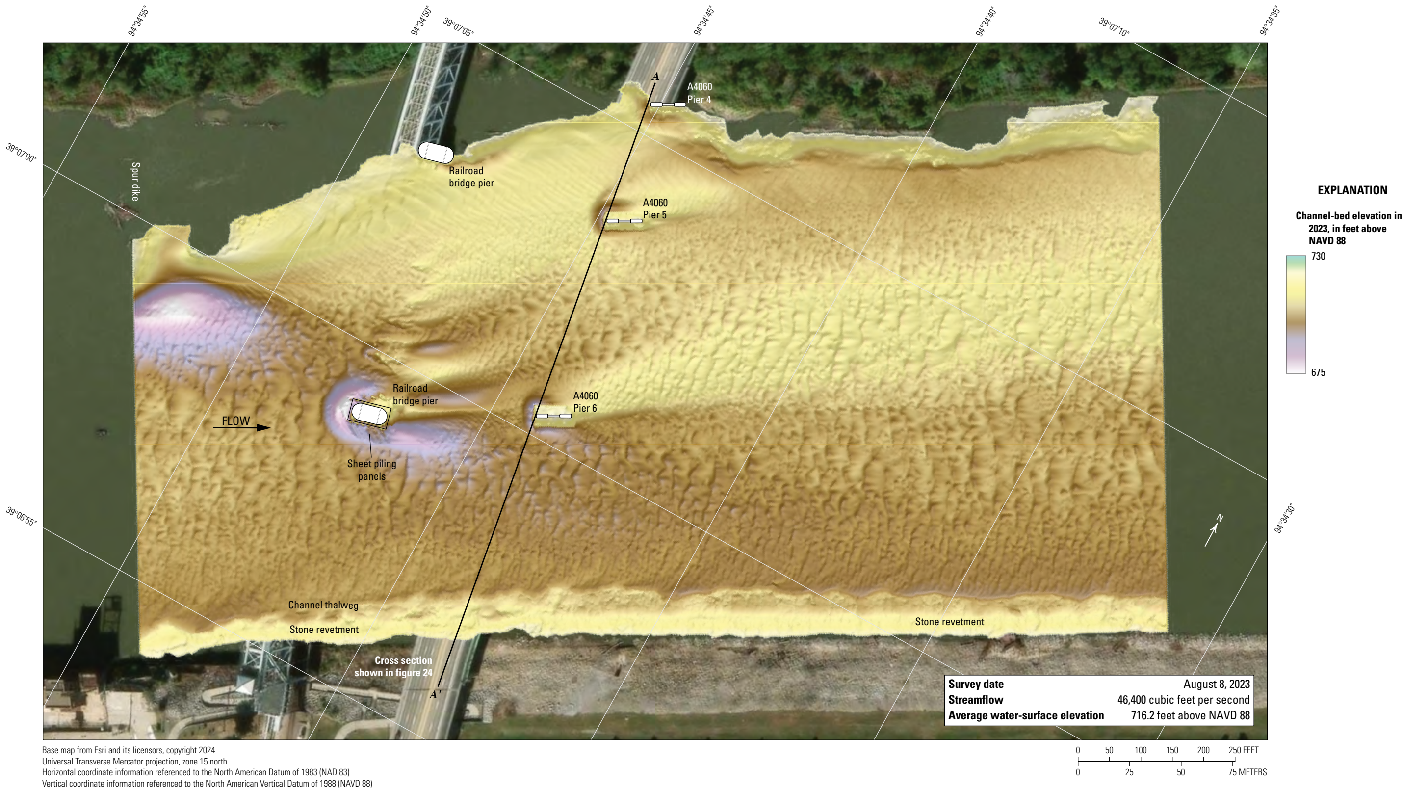
Figure 22. Map showing bathymetric survey of the Missouri River channel near structure A4060 on State Highway 9 in Kansas City, Missouri. [NAVD 88, North American Vertical Datum of 1988]
