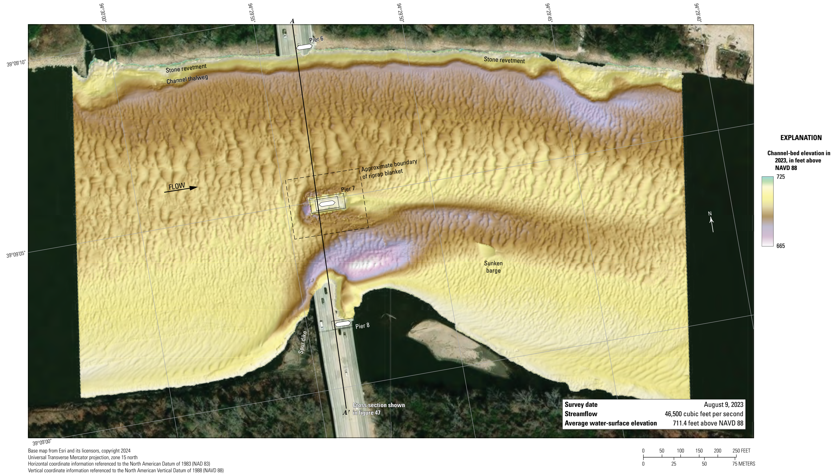
Figure 45. Map showing bathymetric survey of the Missouri River channel near structure A0767 on Interstate 435 in Kansas City, Missouri. [NAVD 88, North American Vertical Datum of 1988]
