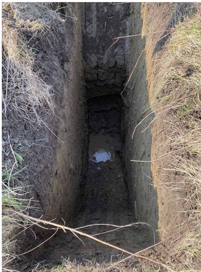
Figure 27. Photographs showing test pits in the proposed offline settling basin area in the Tully Valley, Onondaga County, New York: A , contact between brown silty clay with pebbles and cobbles and gray silty clay at 5 feet (ft) below land surface in test pit OD1999 and B , groundwater seepage pooling in bottom of test pit OD1998. The test pits at their maximum depth (10 ft) were about 3 ft long and 1 ft wide. Photographs by William M. Kappel, U.S. Geological Survey. (Location of test pits shown on fig. 4 .)
