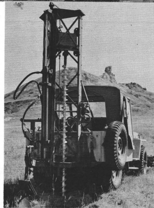
Figure 25.--Jeep-powered auger used in S. Dak. by the Geological Survey to obtain unweathered samples of radioactive lignite.
