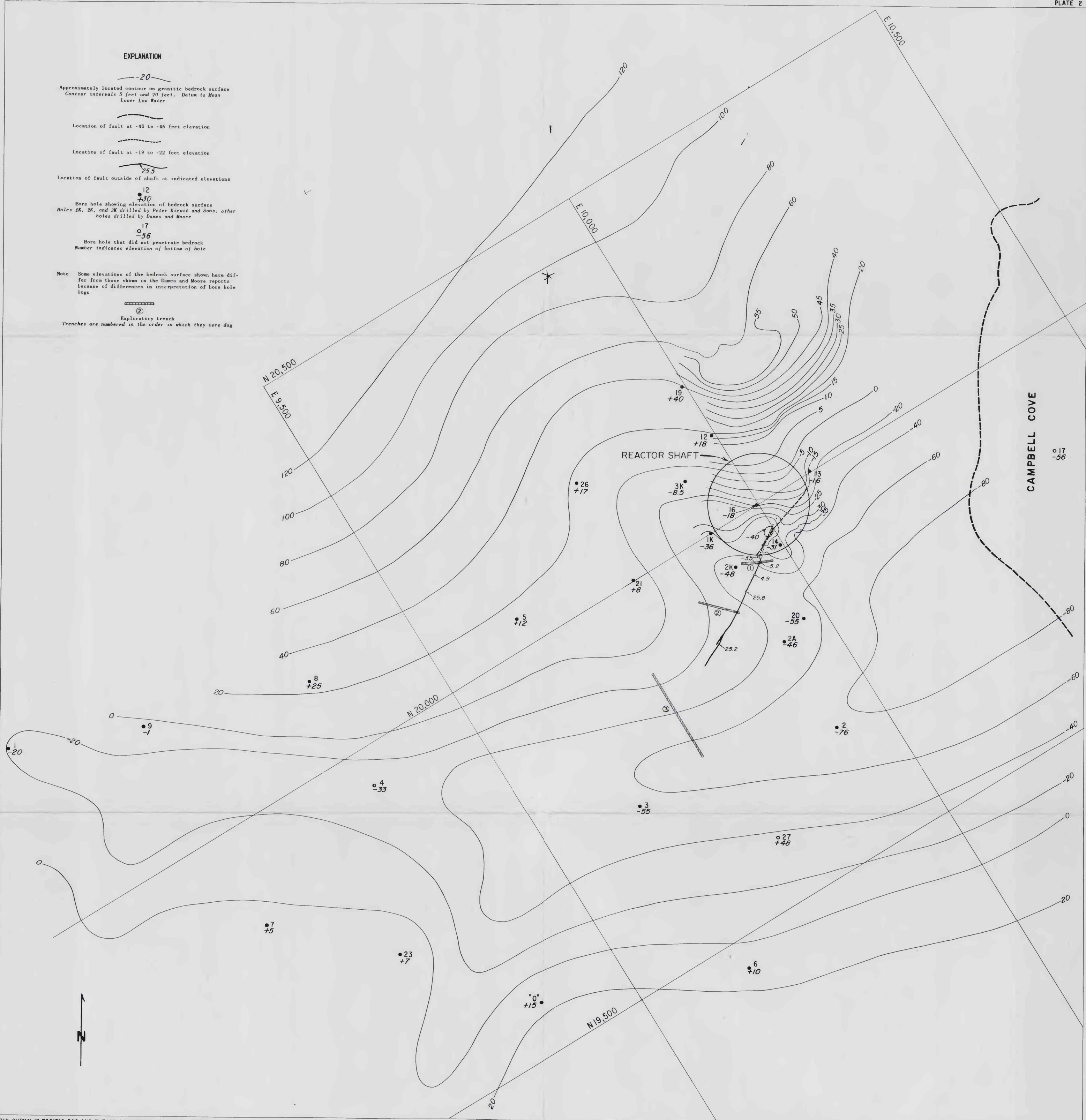
MAP SHOWING CONTOURS ON THE BEDROCK SURFACE, REACTOR SHAFT, SHAFT FAULT, AND EXPLORATORY TRENCHES
