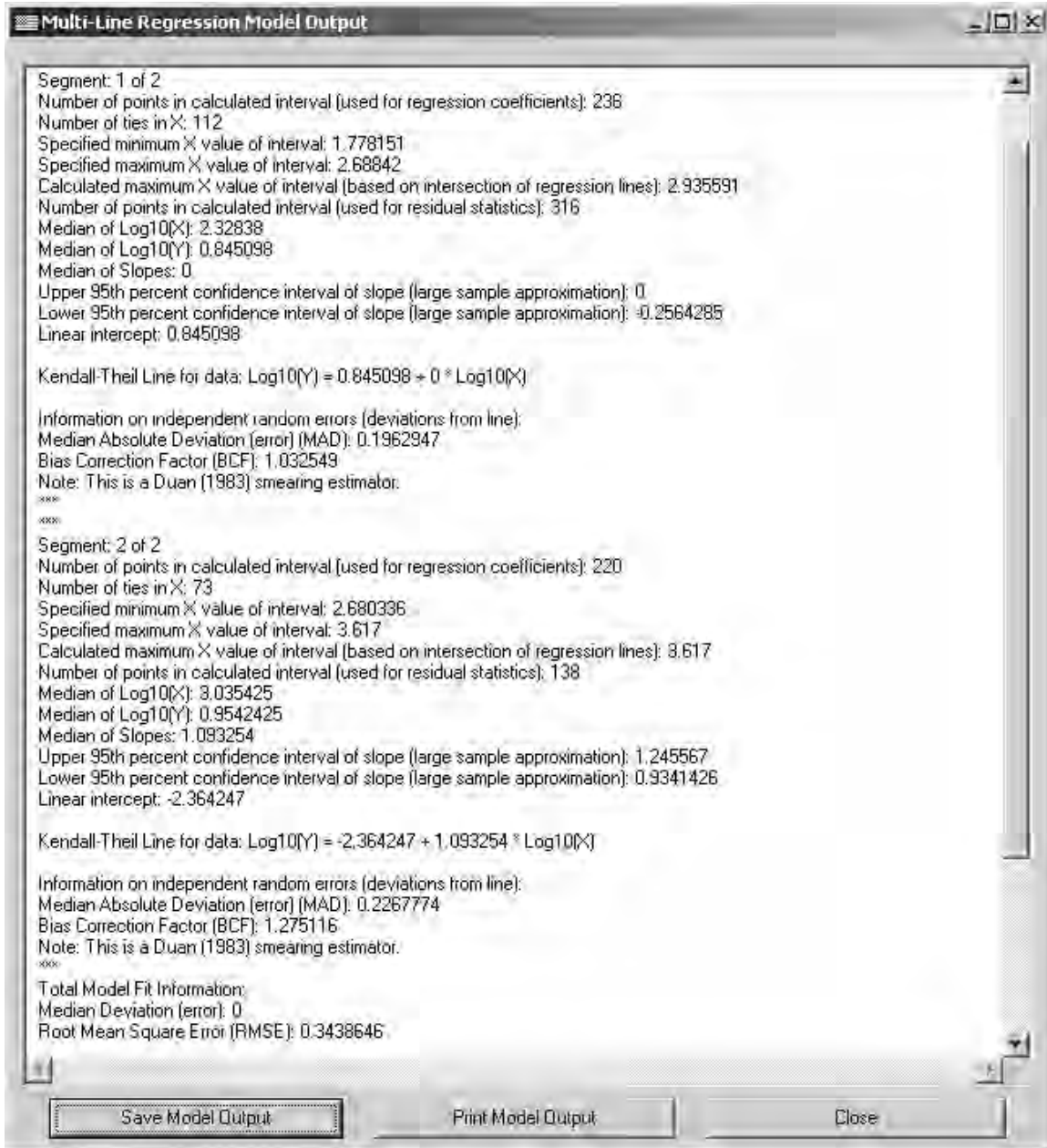
Figure 16. Example of the Kendall-Theil Robust Line multisegment model results screen. This screen provides regression statistics and allows the user to save and print multisegment model results.
