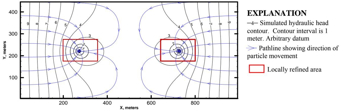
**Figure 3.** Example of grid refinement around two areas of pumping within a coarse-grid model. The system was designed to have a symmetric flow field.
