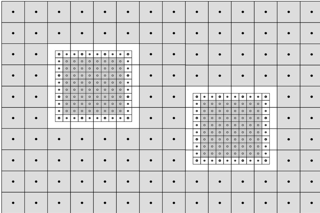
**Figure 2.** Schematic of a coarse grid with two areas of local grid refinement separated by two parent grid cells. At least one parent cell is required between child models.
