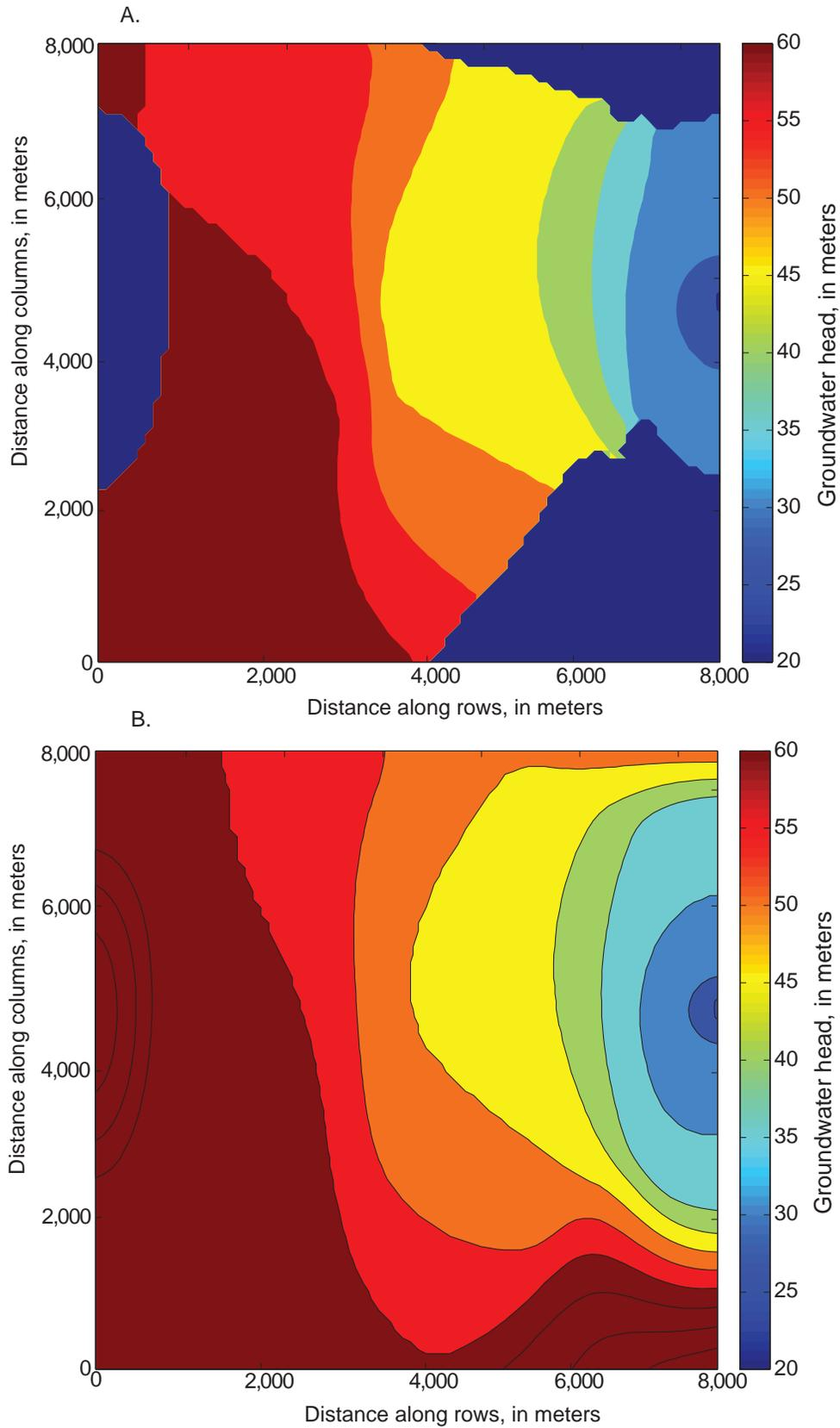
**Figure 11.** Distribution of heads for problem 3 with higher recharge values (fig. 10), (A) MODFLOW-2005, and (B) MODFLOW-NWT. The dark blue regions in (A) indicate cells that are dry in the MODFLOW-2005 simulation, whereas all cells have heads greater than 2 mm above the cell bottom in the MODFLOW-NWT simulation.
