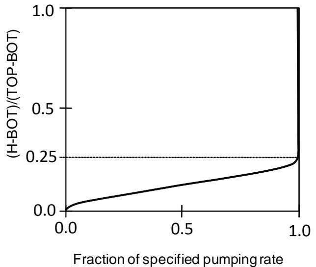
**Figure 4.** Curve used to smoothly reduce specified pumping to zero when cell dewateres,  $\Phi = 0.25$ .
