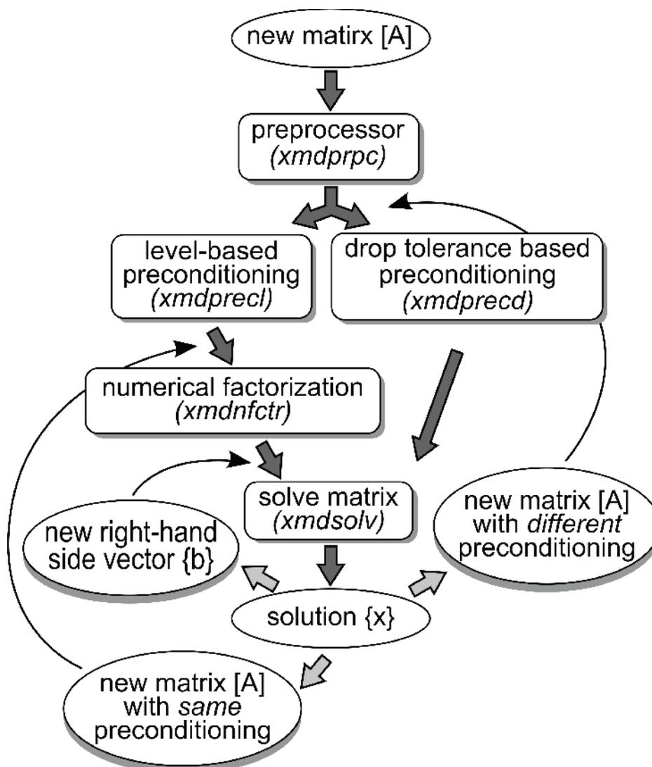
**Figure C1.** Sequence of calling subroutines in  $\chi$ MD.
