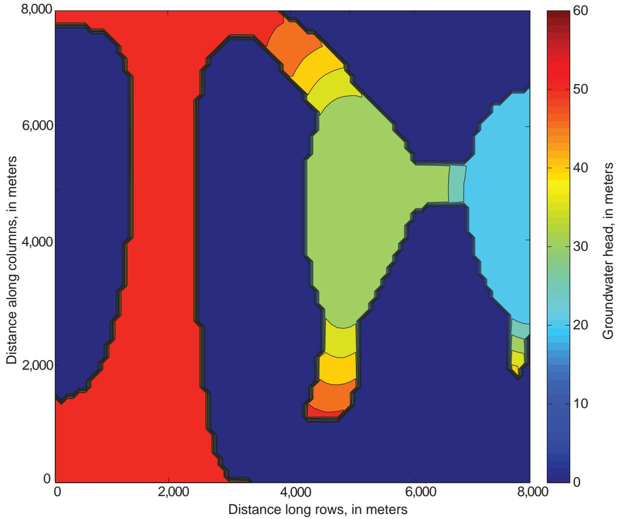
**Figure 14.** Distribution of groundwater heads calculated by MODFLOW-NWT for problem 3 with lower recharge values ([fig. 10](#)). The dark blue regions indicate cells that have heads less than 2 mm above the cell bottom.
