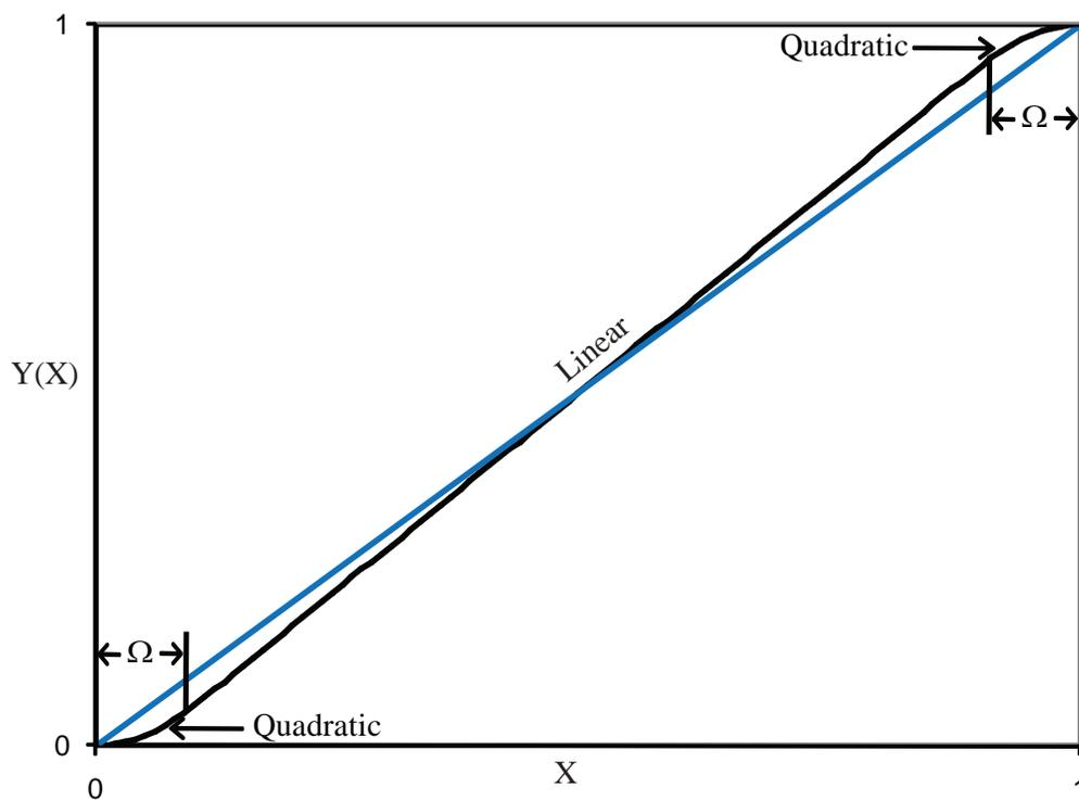
**Figure 1.** Combined quadratic and linear functions used to smooth conductance and storage in MODFLOW-NWT (black), and a linear function that is used by MODFLOW-2005 (blue).  $X$  is the saturated thickness divided by the cell thickness,  $Y$  is the value of the smoothing function, and  $\Omega$  is the interval of  $X$  where the quadratic equation is applied, and is equal to 0.1 in this example (NWT input file variable THICKFACT).
