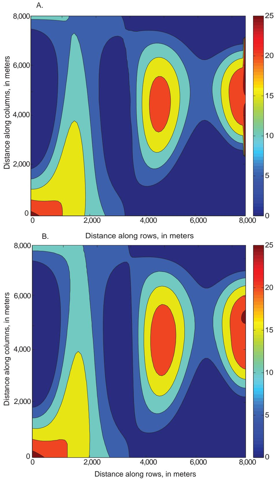
**Figure 13.** Distribution of saturated thickness for problem 3 with higher recharge values (fig. 10). (A) MODFLOW-2005, and (B) MODFLOW-NWT. Units used for saturated thickness are meters above cell bottom.
