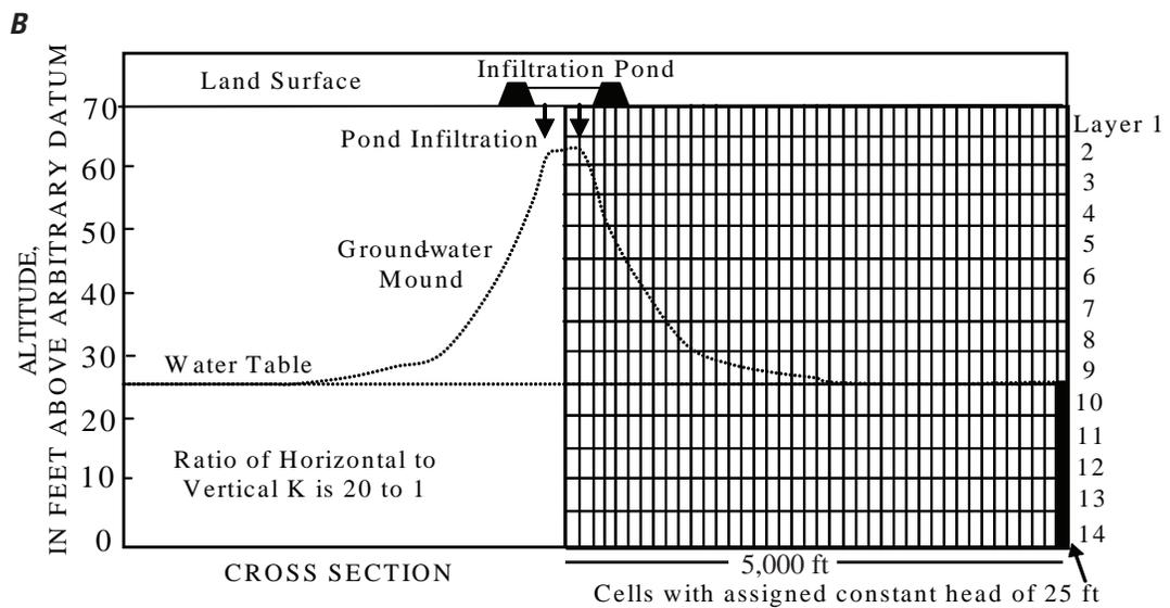
**Figure 7.** Diagrams showing (A) plan view of model, and (B) cross-section of model used for model comparison.
